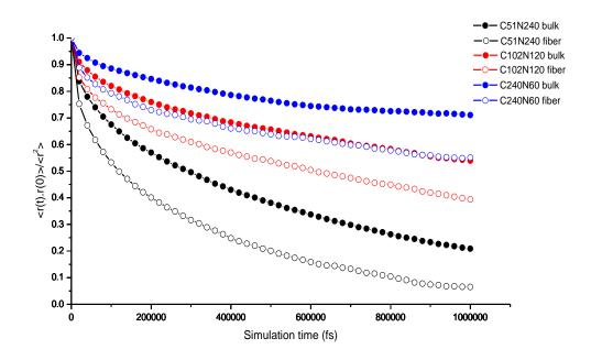
**Figure 7** Decorrelation function of the end-to-end vector of PE molecules as function of simulation time.
