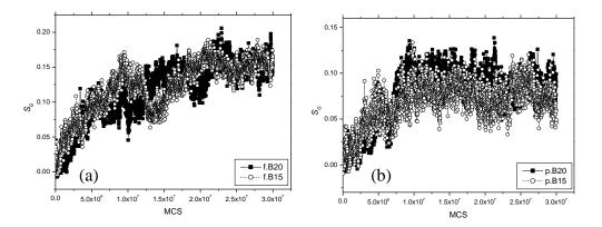
**Figure 4.43** The global orientation order parameter,  $S_G$ , as a function of MCS after quenching from 509 to 298 K (a) nanofiber and (b) nanoparticle.
