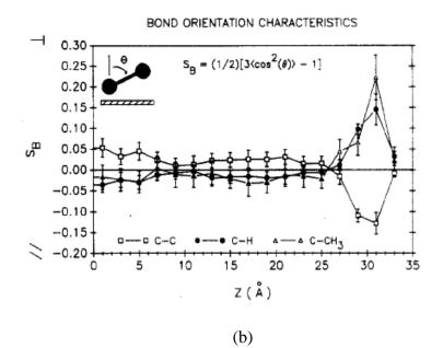
**Figure 2.2** (a) The local mass density distribution at a glassy polymer vacuum interface. (b) Local order parameter for C-C, C-H, and C-CH<sub>3</sub> bonds as a function of distance from the film midplane (Mansfield and Theodorou, 1990).
