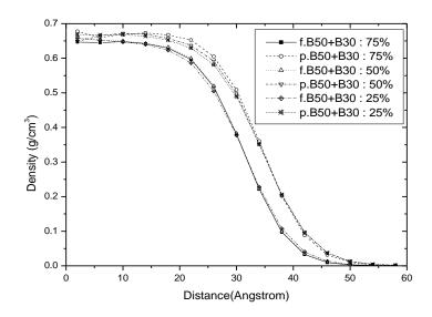
**Figure 4.28** Effect of composition on total density profile of bidisperse PE naofiber and nanoparticle in B50+B30 system.
