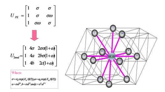
Figure 2 Schematic representation of the first shell contacts on the 2nnd lattice.
