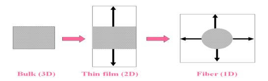
**Figure 3** Elongation method to generate a new cohesive polymer structure from bulk  $(3D) \rightarrow$  Thin film  $(2D) \rightarrow$  Fiber (1D). The views of the film and fiber are in the plane of the film and along the axis of the fiber.
