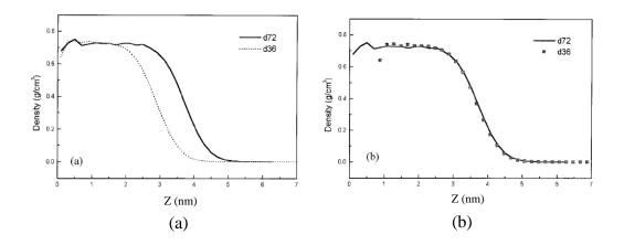
**Figure 2.7** (a) Radial density profiles as a function of distance from the center of mass of the nanoparticle. (The bulk density is ~ $0.7 \text{ g.cm}^{-3}$ ). In (b) the data for d36 are moved to the right by 0.10 nm to show the superimposition on the d72 curve (Vao-soongnern *et al.*, 2001).
