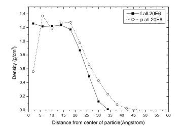
Figure 3.40 Comparison of crystal density profile between nanofiber and nanoparticle at  $3 \times 10^7$  MCS.
