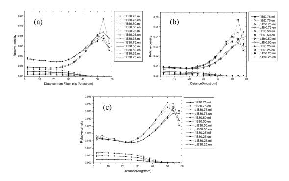
**Figure 4.29** The relative density of middle bead and end bead of bidisperse PE in B50+B30 system (a) nanofiber (b) comparison between B50 nanofiber and nanoparticle and (c) comparison between B30 nanofiber and nanoparticle.
