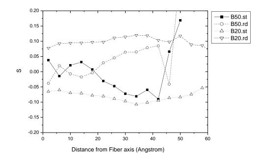
**Figure 4.7** The orientation of the largest and smallest principal moment to fiber axis after equilibration of monodisperse B50 and B20 PE nanofibers.
