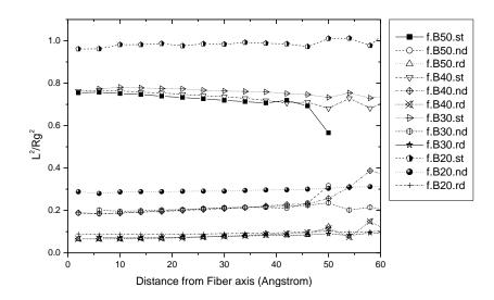
**Figure 4.14** The principal moment of chains (normalized by  $R_g^2$ ) as a function of radial displacement of the center of mass from fiber axis of monodisperse PE nanofibers.
