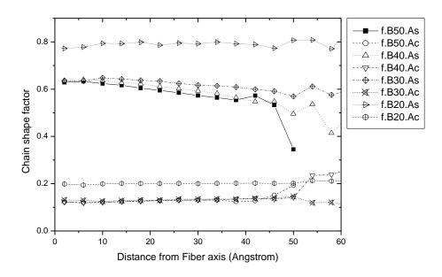
**Figure 4.12** The change in chain shape (asphericity and acylindricity) as a function of radial displacement of the center of mass from fiber axis of monodisperse PE nanofibers.
