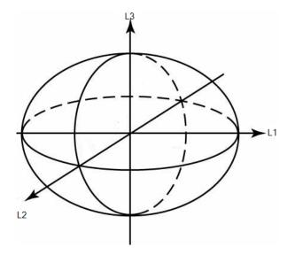
**Figure 4.6** The ellipsoid was defined of the principal components L3 < L2 < L1 for PE molecule.
