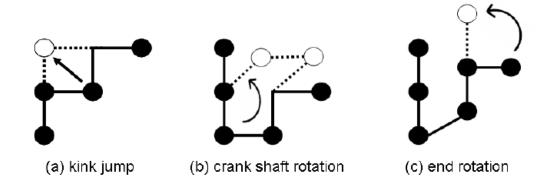
Figure 3.1 Basic elementary moves based on the standard Verdier-Stockmayer type model.
