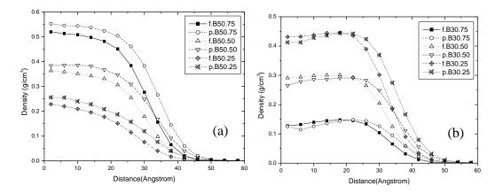
**Figure 4.27** Comparison the density profile of B50+B30 between bidisperse PE nanofiber and nanoparticle system (a) long chain (B50) and (b) mixed chain.
