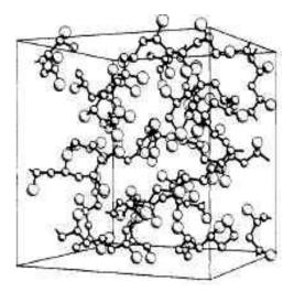
**Figure 2.1** "Relaxed" model structure in detailed mechanical equilibrium. The small spheres denote skeletal carbon atoms, the large spheres indicate methyl groups, and hydrogen atoms have been omitted for clarity (Theodorou and Suter, 1985).
