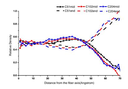
Figure 5 Radial density profiles for mid/end beads of monodisperse PE.
