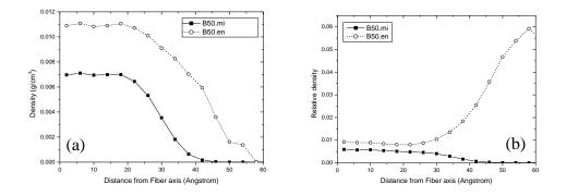
**Figure 4.3** (a) Radial density profiles for mid/end beads of monodisperse PE B50 at 509 K. (b) result after normalization by the bulk density.
