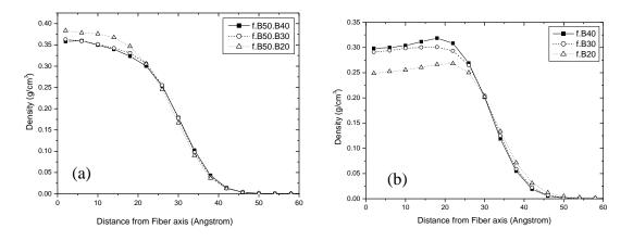
**Figure 4.17** The density profile of bidisperse PE nanofibers which B50 composition is 50% (a) B50 and (b) B40, B30, B20.
