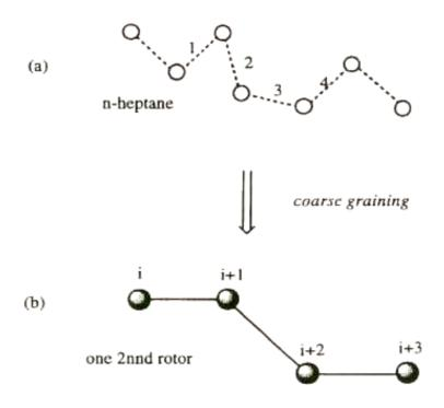
**Figure 3.6** The coarse graining of n-heptane with 4 rotors to a single rotor in 2nnd lattice: (a) n-heptane (b) 2nnd chain equivalent to n-heptane.
