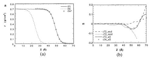
**Figure 2.3** (a) Density profiles of two PE films at 509 K as a function of the distance from the center of mass in the Z direction. (b) Orientation of the coarse-grained 2nnd bonds with the Z-axis (Doruker and Mattice, 1998).
