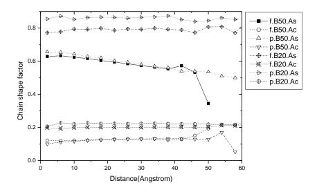
**Figure 4.13** Comparison of the change in chain shape (asphericity and acylindricity) as a function of radial displacement of the center of particle of monodisperse PE nanoparticles.
