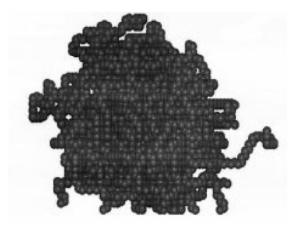
**Figure 2.6** Illustration of the smaller amorphous PE nanoparticle composed of 36 coarse-grained chains of  $C_{100}H_{204}$  from the 2nnd lattice simulation. Only the backbone carbon atoms are shown (Vao-soongnern *et al.*, 2001).
