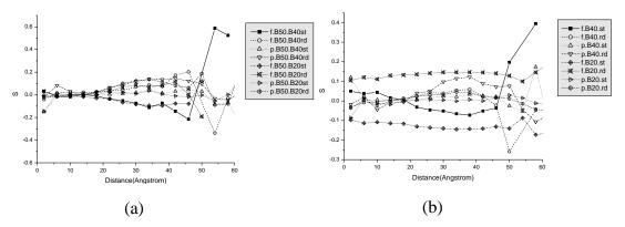
**Figure 6** Comparison of the orientation of the largest and smallest principal moment to axis after equilibration of nanofibers and nanoparticles (a) B50 and (b) B40 and B20.
