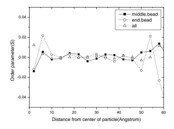
**Figure 4.4** The orientation of chords (mid-, end- and all) of monodisperse B30 PE nanoparticle.
