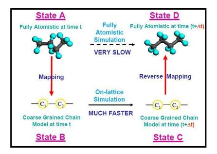
**Figure 1** Schematic representation of the comparison between two alternative pathways: fully atomistic off-lattice and coarse-grained on lattice simulations.
