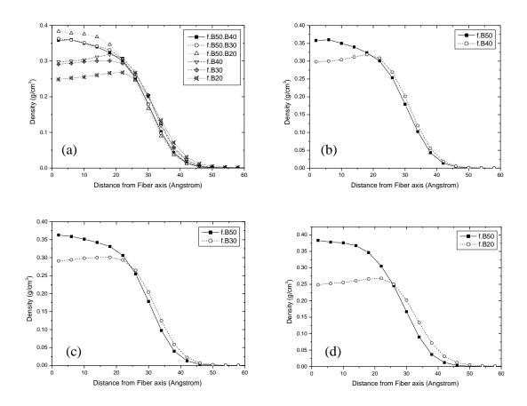
**Figure 4.16** The density profile of bidisperse PE nanofibers which B50 composition is 50% (a) total density of short and long chain, (b) B50+B40, (c) B50+B30 and (d) B50+B20.
