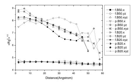
Figure 4.11 Comparison of the change in the  $R_g$  components as a function of radial displacement of the center of mass between monodisperse PE nanofibers and nanoparticles.
