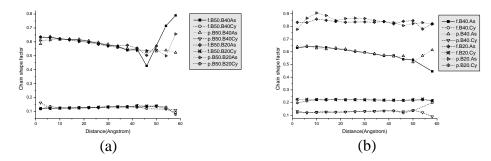
**Figure 9** Comparison of the change in molecular shape (asphericity and acylindricity) as a function of radial displacement of the center of mass (a) B50 nanofiber and nanoparticle (b) B40 and B20 nanofiber and nanoparticle.
