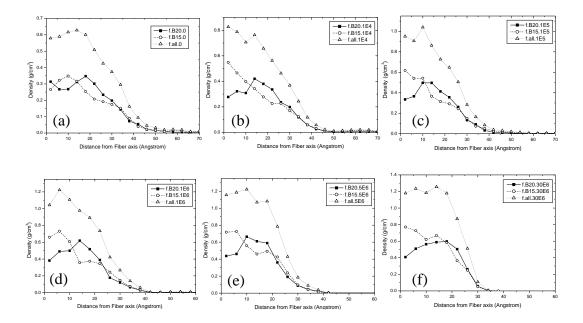
**Figure 4.36** Density profile of B20 and B15 nanofiber normal to the fiber axis after quenching from 509 K to 298 K and simulation at 298 K (a) 0, (b)  $1 \times 10^4$ , (c)  $1 \times 10^5$ , (d)  $1 \times 10^6$ , (e)  $5 \times 10^6$  and (f)  $3 \times 10^7$  MCS.
