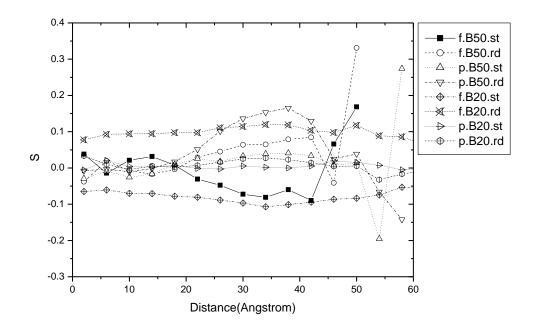
**Figure 4.8** Comparison of the orientation of the largest and smallest principal moment to center of particle between monodisperse PE nanofibers and nanoparticles.
