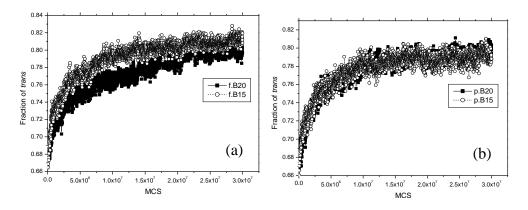
**Figure 4.41** The fraction of C-C bonds that are in the *trans* state as a function of MCS after quenching from 509 to 298 K (a) nanofiber and (b) nanoparticle.
