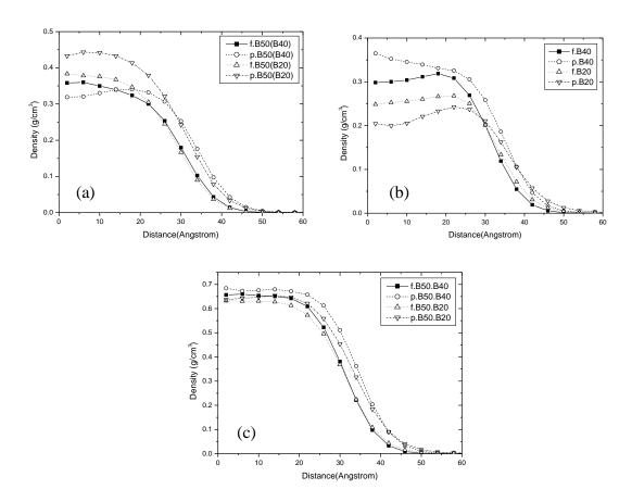
**Figure 4.18** Comparison of density profile of bidisperse PE between nanofibers and nanoparticle which B50 composition is 50% (a) B50 and (b) B40, B30, B20 and (c) total density.
