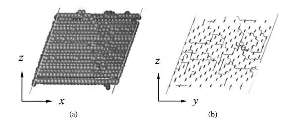
**Figure 2.8** Snapshot of the internal structure of the final conformation of an atypical thin film at 298 K, represented by (a) all carbon atoms, viewed along the y axis, and (b) all C-C bonds, viewed perpendicular to the x axis (along the long axis of the ordered chains) (Xu and Mattice, 2002).
