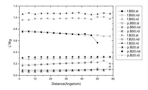
**Figure 4.15** Comparison of the principal moment of chains (normalized by  $R_g^2$ ) as a function of radial displacement of monodisperse PE nanofiber and nanoparticle.
