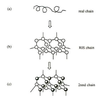
**Figure 3.3** Example of the mapping of a real chain into lattice by coarse graining. The degree of coarse graining increases from (a) to (c). (a) continuous space, (b) space available with a single bond length, tetrahedral bond angle, and  $\phi = 180^{\circ}$ ,  $\pm 60^{\circ}$ , (c) rejection of alternate sites from (b).
