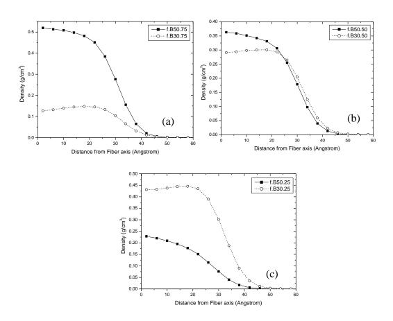
**Figure 4.26** Density profiles of bidisperse PE nanofiber in the system of B50+B30 which the composition of B50 is (a) 75% (b) 50% and (c) 25%.
