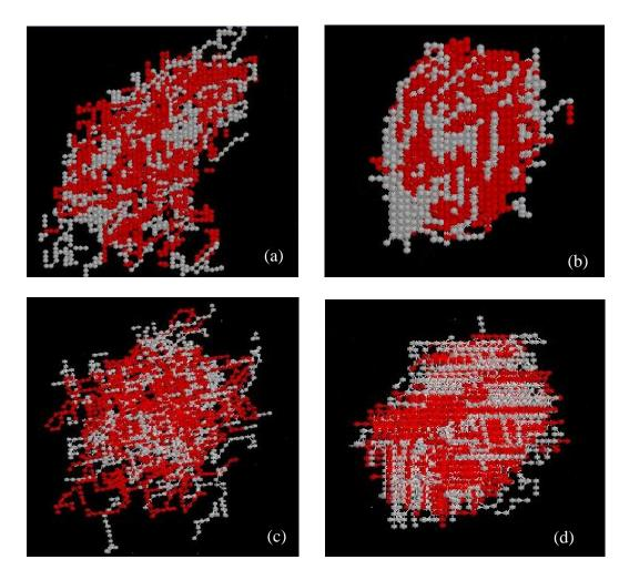
**Figure 4.42** The structure of (a) nanofiber (0 MCS), (b) nanofiber (30 MCS), (c) nanoparticle (0 MCS) and (d) nanoparticle (30 MCS) (red = B20, gray = B15).
