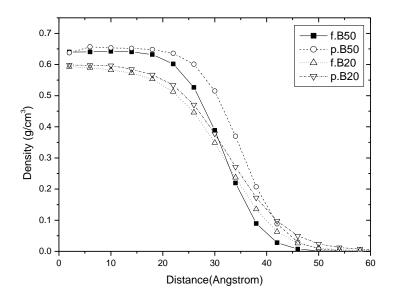
**Figure 4.2** Comparison of density profile between monodisperse B50 and B20 PE nanofiber and nanoparticle at 509 K.
