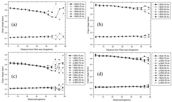
**Figure 4.34** Changing in shape (asphericity and acylindricity) as a function of radial displacement of the center of mass in B50+B30 system (a) B50 nanofiber, (b) B30 nanofiber, (c) B50 nanofiber and nanoparticle and (d) B30 nanofiber and nanoparticle.
