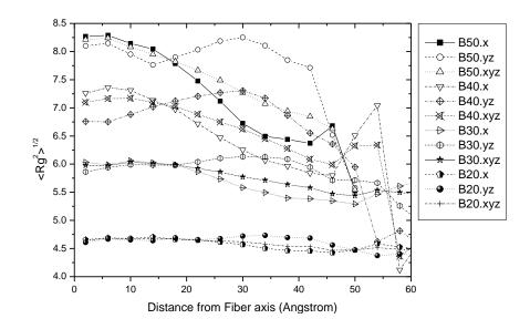
Figure 4.10 The change in the  $R_g$  components as a function of radial displacement of the center of mass from fiber axis of monodisperse PE nanofibers.
