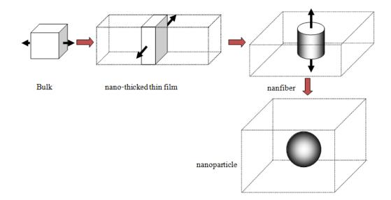
**Figure 3.8** The method to generate a new cohesive polymer structure from bulk (3D)  $\rightarrow$  nano-thicked thin film (2D)  $\rightarrow$  nanofiber (1D)  $\rightarrow$  nanoparticle(0D).
