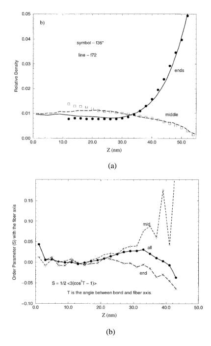
**Figure 2.5** (a) Normalized radial density profiles for mid/end beads for f36 and f72 of C99 at 509 K. (b) The orientation of chords (mid-, end- and all) (Vao-soongnern *et al.*, 2000).
