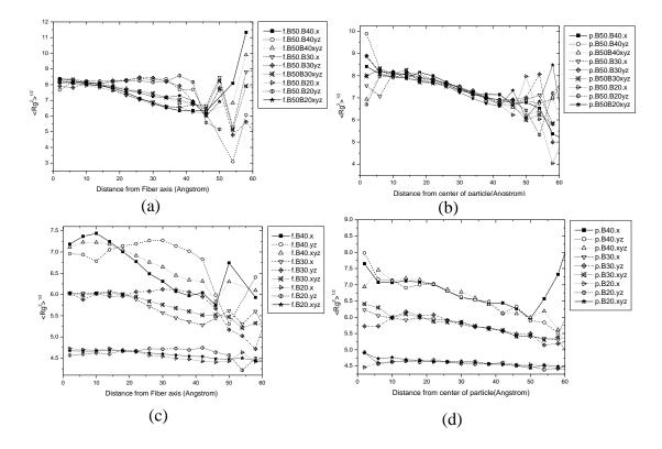
**Figure 4.23** Comparison of the changing in the  $R_g$  components to center of mass after equilibration between bidisperse PE nanofibers and nanoparticles which B50 composition is 50% (a) B50 nanofiber (b) B50 nanoparticle (c) B40, B30 and B20 nanofiber and (c) B40, B30 and B20 nanoparticle.
