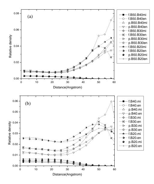
**Figure 4.19** The relative density of middle bead and end bead of bidisperse PE nanofibers and nanoparticle which B50 composition is 50% (a) B50 and (b) B40, B30, B20.
