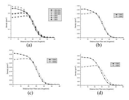
**Figure 2** The density profiles of bidisperse PE nanofiber (a) total density, (b) component in B50+B40, (c) B50+B30 and (d) B50+B20 systems.
