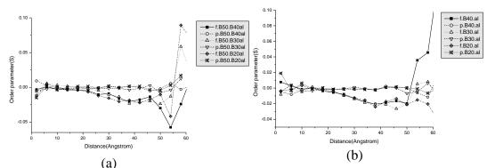
**Figure 5** Comparison of the orientation of chords (all) of nanofibers and nanoparticles (a) B50 and (b) B40, B30, B20.
