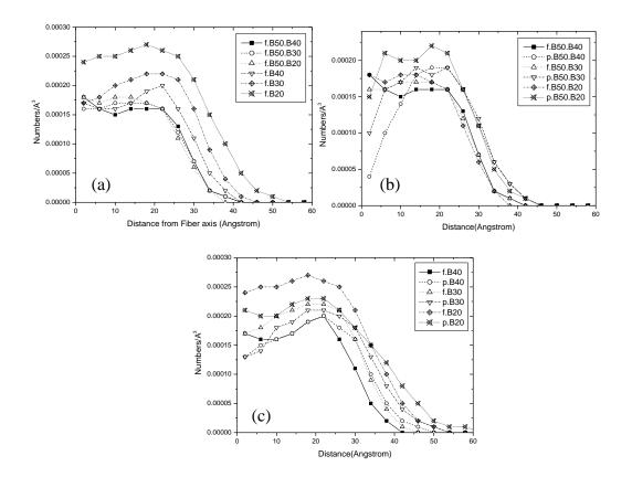
**Figure 4.22** The center of mass distribution as a function of radial displacement bidisperse PE systems which B50 composition is 50% (a) nanofiber (b) the long chain(B50) nanofiber and nanoparticle (c) the mixed chain nanofiber and nanoparticle.
