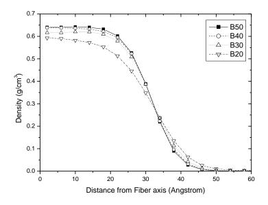
**Figure 4.1** Radial density profiles of monodisperse B50, B40, B30 and B20 PE nanofibers at 509 K.
