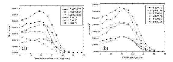
**Figure 4.32** The center of mass distribution as a function of radial displacement in B50+B30 system (a) PE nanofiber (b) PE nanofiber and nanoparticle.
