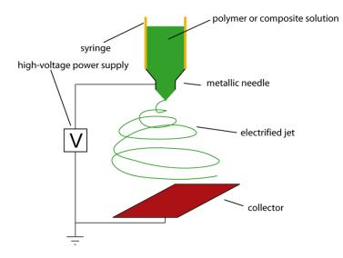
**Figure 1.4** Schematic representation of nanofiber formation by Electrospinning process (Wikimedia Commons, 2009).
