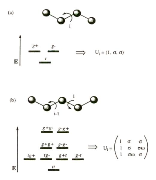
**Figure 3.5** The rotational states of a linear chain and corresponding statistical weights (a) independent bond (b) interdependent bond.
