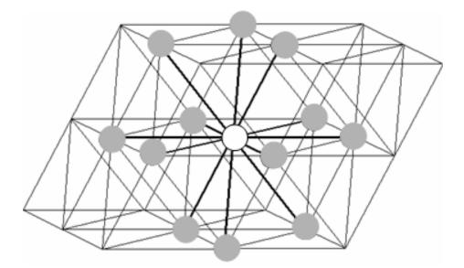
**Figure 3.4** The 2nnd lattice. The gray spheres represent the possible twelve coordination lattice sites around a central bead (open circle).
