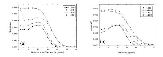
**Figure 4.9** The center of mass distribution as a function of radial displacement (a) mono disperse nanofiber (b) comparison between monodisperse PE nanofiber and nanoparticle (B50 and B20).
