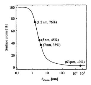
**Figure 1.2** The percentage of surface atoms changes with the palladium cluster diameter (Nützenadel *et al.*, 2000).
