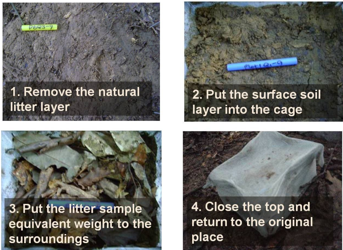
Picture 4 Setting of fine cages.
