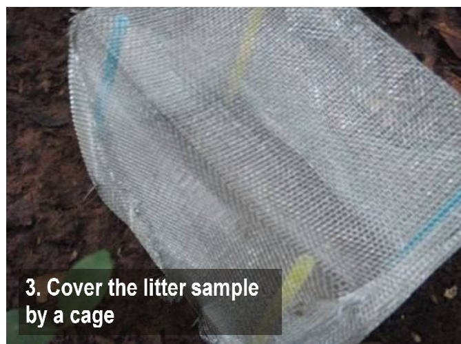
Picture 3 Setting of coarse cages.
