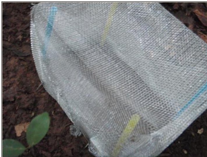
Picture 2 Coarse and open-bottom cage General mesh (2.0 mm) Allowance of termites.
