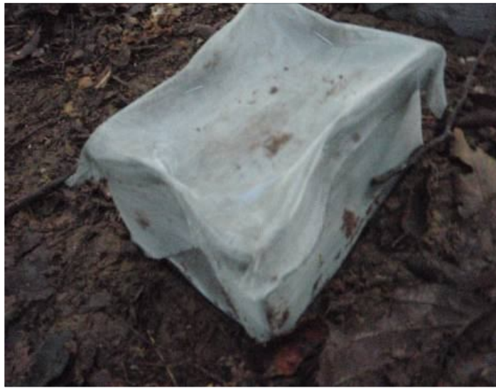
Picture 1 Fine and enclosed cage Termimesh® (0.2 mm) No allowance of termites.
