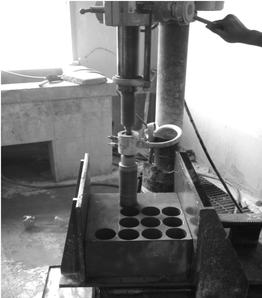
Figure 3.2 Laboratory core drilling of PK sandstone. The core drilling machines (model SBEL 1150) are used to drill core specimens using diamond impregnated bit with diameters of 54 mm and 37 mm.
