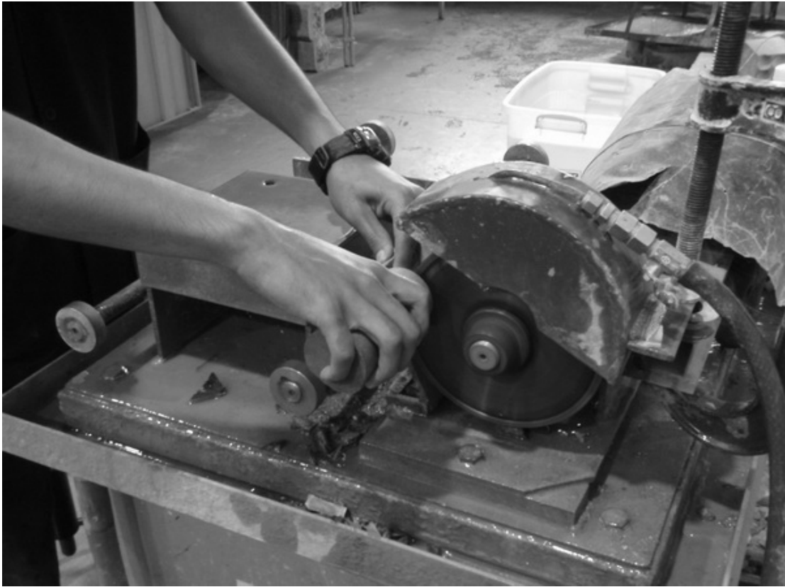
Figure 3.3 A core specimen of PK sandstone is cut by a cutting machine.
