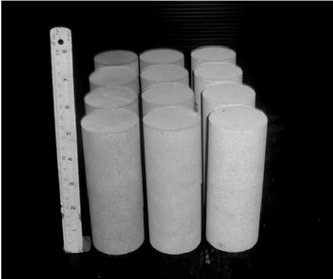
Figure 3.4 PK, PP and PW sandstones specimens prepared for the uniaxial compressive strength test have 54 mm in diameter and with L/D ratio of 2.5
