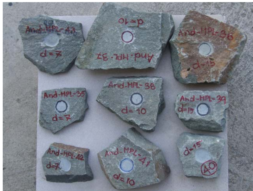
Figure 3.2 Some prepared rock specimens of porphyritic andesite for MPL Tests.
