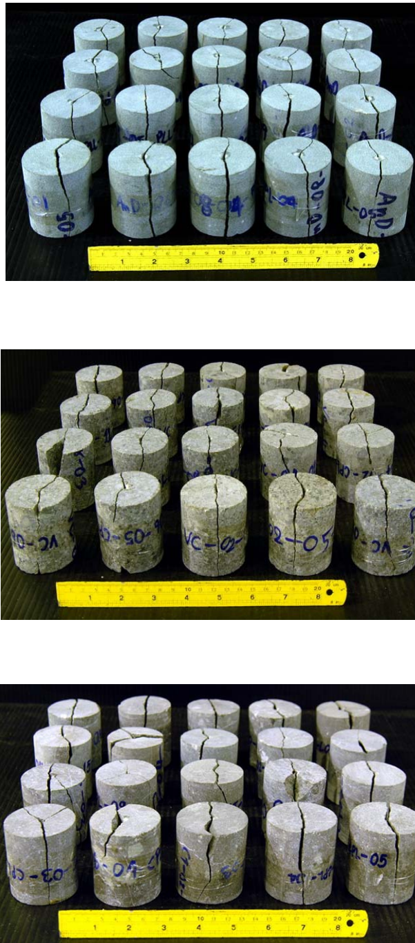
Figure 4.23 Post-Test rock specimens from conventional point load strength index tests. (a). porphyritic andesite (b). tuffaceous sandstone, and (c). silicified tuffaceous sandstone.
