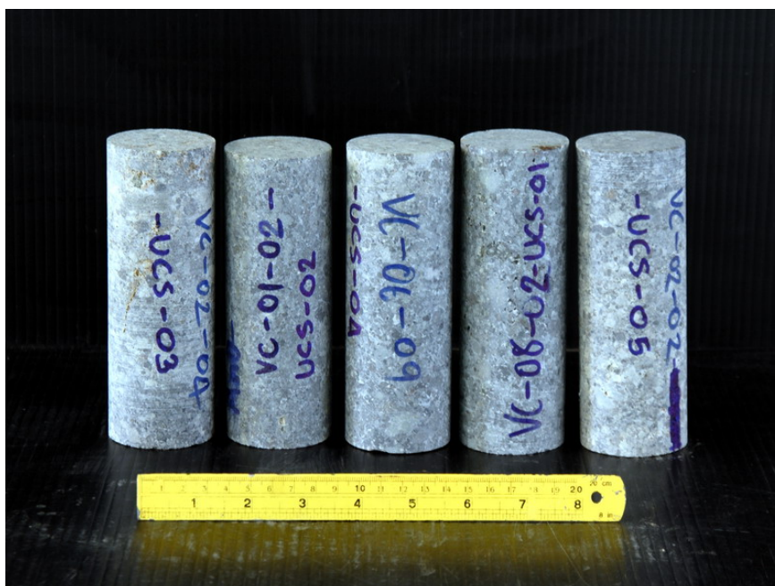
Figure 4.2 Pre-test samples of tuffaceous sandstone for UCS test
