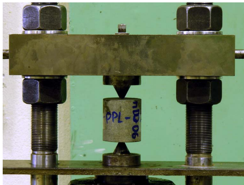
Figure 4.22 Conventional point load strength index test arrangement.
