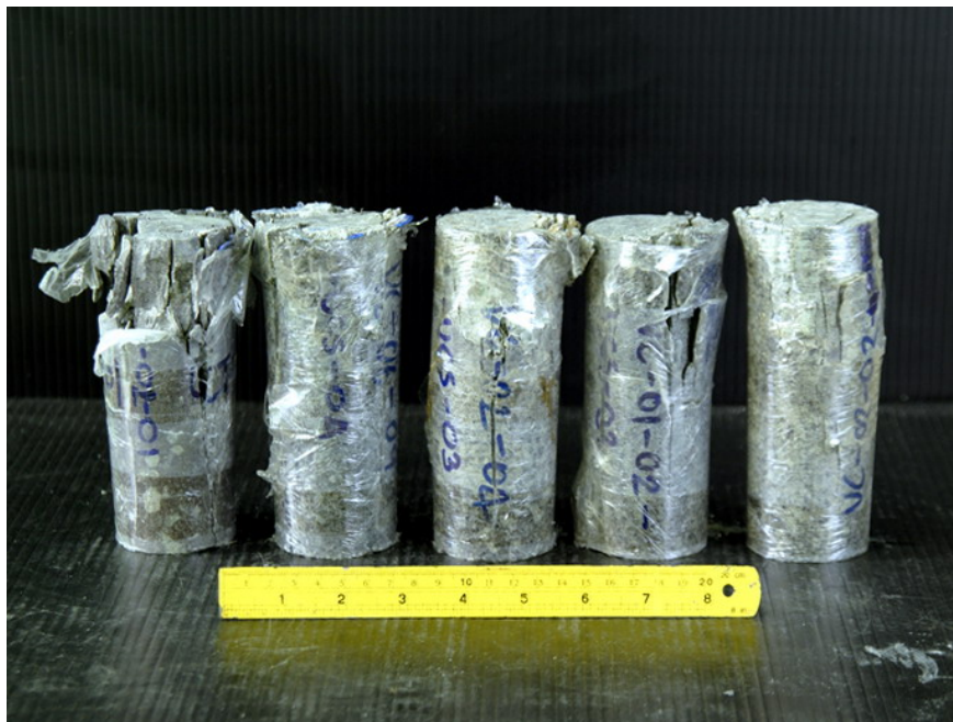
Figure 4.6 Post-test rock samples of tuffaceous sandstone from UCS test
