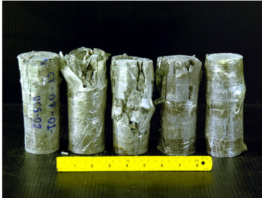
Figure 4.7 Post-test rock samples of silicified-tuffaceous sandstone from UCS
