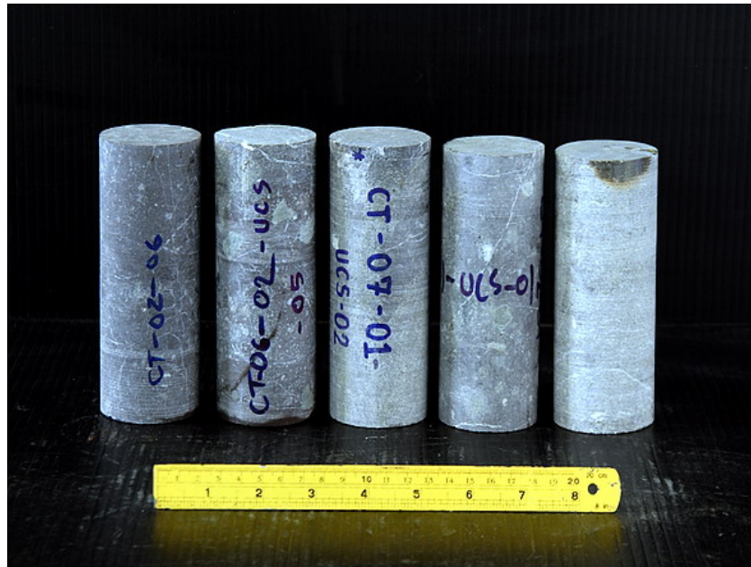
Figure 4.3 Pre-test samples of silicified tuffaceous sandstone for UCS test
