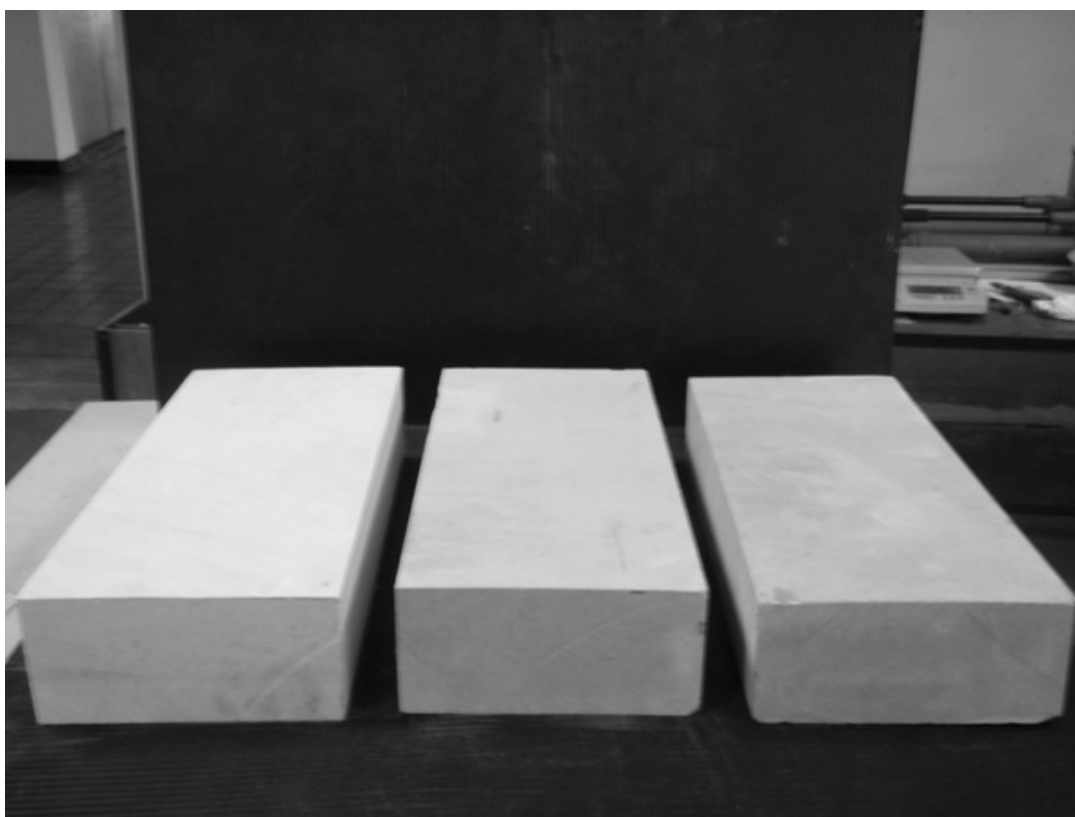
Figure 3.1 Sandstones blocks with nominal size of 10 cm x 20 cm x 40 cm are collected from Saraburi province. Left: Phra Wihan, Middle: Phu Phan and Right: Phu Kadung.
