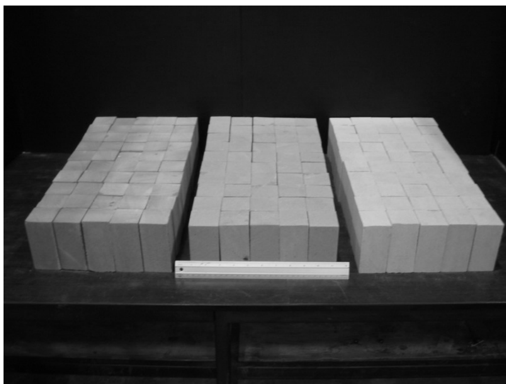
Figure 3.2 Sandstone specimens prepared for true triaxial stress. Left: Phu Kadung, Middle: Phu Phan and Right: Phra Wihan.
