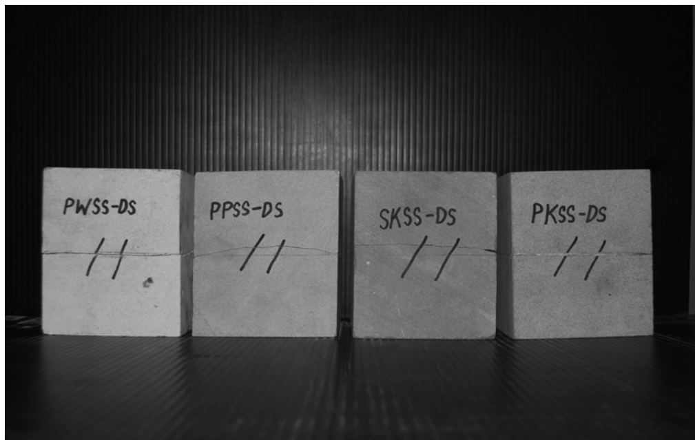
Figure 3.1 Some sandstone specimens prepared for falling head test under normal and shear stresses.
