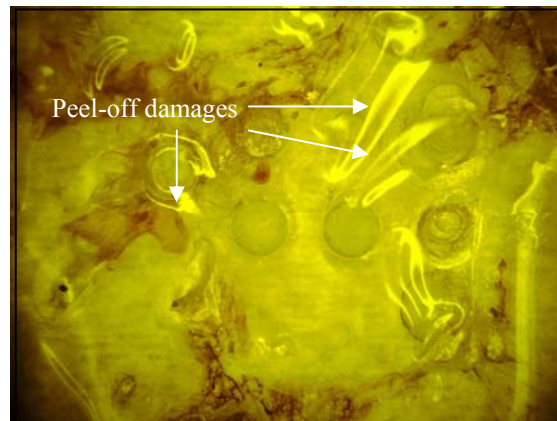
Figure 5.6 Peel-off damages of the PDMS membrane after testing.
