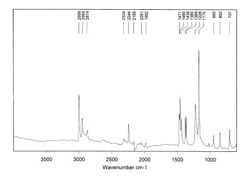
Figure B6.5 The IR spectrum for the AIBN ligand.
