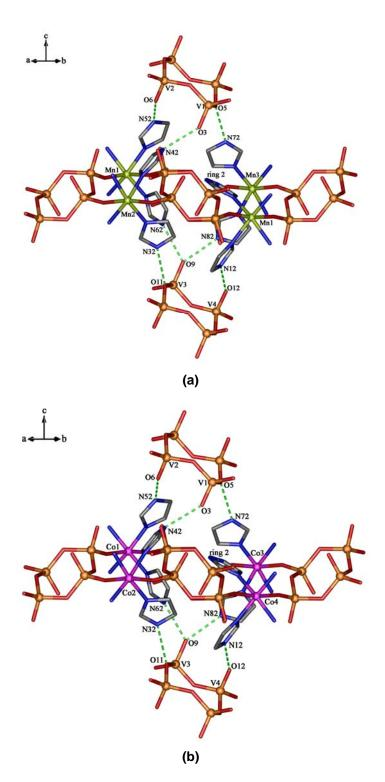
Figure 7.9 Hydrogen bonds about the pseudo inversion centers 3/4, 1/4, 1/2 for the  $I4_1/a$  structure at 100(2) K of (a) 7b, (b) 7c, and 0, 1/2, 1 for the  $P4_2/n$  structure at 295(2) K of (c) 7b, (d) 7c. The 1:1 disorder of the  $P4_2/n$  structure is not shown.
