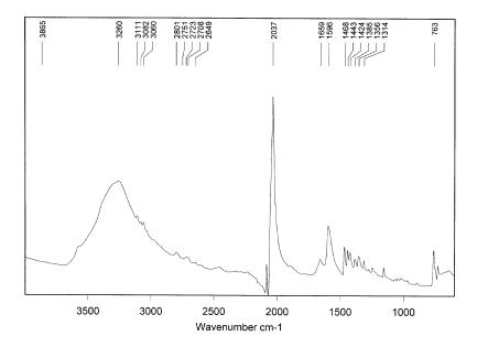
**Figure B3.3** The IR spectrum for  $K_2[Fe^{II}(2,2'-bipy)(CN)_4]\cdot 3H_2O$ .
