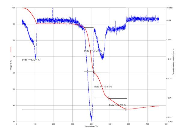
Figure 5.13 TGA (red) and DTA (blue) profiles for 5a.
