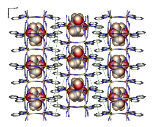
**Figure 3.4** Packing diagram of **3a** viewed along the *c* axis showing  $\pi \cdots \pi$  interactions between the 2-D corrugated sheets. Methanol molecules are represented as space-filling models.
