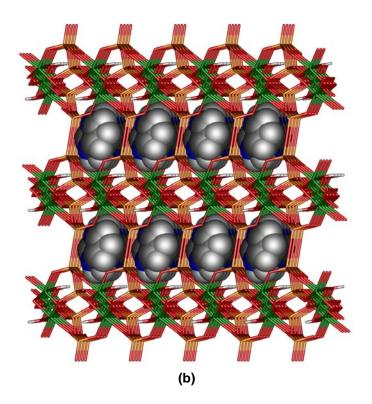
Figure 7.4 (a) Polyhedral and ball-and-stick representation of 7a viewed approximately along the *a* axis, and (b) wires/stick and space-filling representation viewed along the *b* axis of 7a. The disordered imidazolium molecules are located in the middle of the channels.
