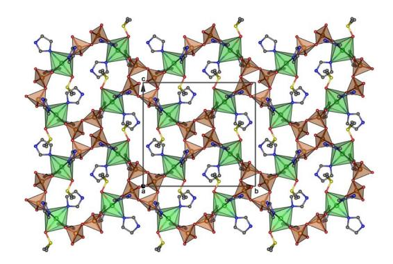
Figure 7.12 Polyhedral representations of single layer of compound 7e, viewed along the crystallographic *a* axis. The layer is at z = 1/2.
