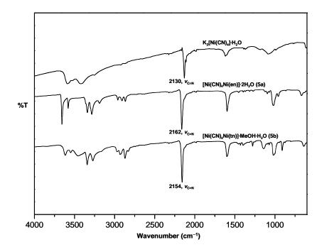
Figure 5.12 ATR-FTIR spectra of  $K_2[Ni(CN)_4]$ ·H<sub>2</sub>O, 5a and 5b.
