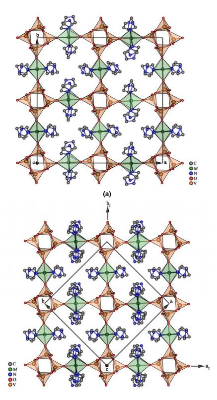
Figure 7.7 Polyhedral representations of single layer of compounds at (a)  $I4_1/a$  and (b)  $P4_2/n$ , viewed along the crystallographic **c** axis. The layers are at z = 1/2 for  $I4_1/a$ , and z = 1 for  $P4_2/n$ .
