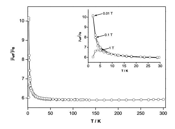
Figure 3.19 Plot of magnetic moment, per [Mn<sup>II</sup>Fe<sup>II</sup>], in fields of 0.01, 0.1 and 1 T for
