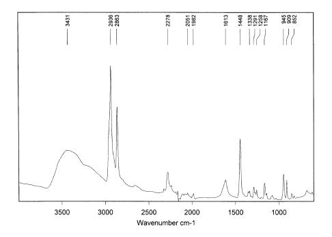
Figure B6.3 The IR spectrum for 6d.
