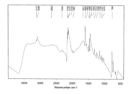
**Figure B3.4** The IR spectrum for  $H[Fe^{III}(2,2'-bipy)(CN)_4] \cdot 2H_2O$ .
