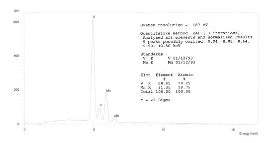
Figure B7.7 The EDX spectrum for 7e.
