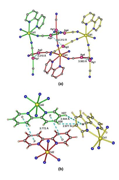
Figure 4.19 Views of a fragment of the alternating nets in 4d showing (a) the Ag…Ag argentophilic and (b) C–H… $\pi$  and  $\pi$ … $\pi$  interactions (dotted lines).
