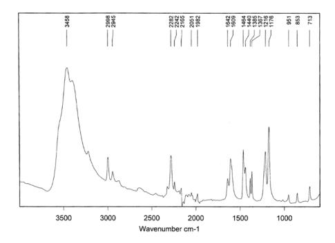
Figure B6.2 The IR spectrum for 6b.
