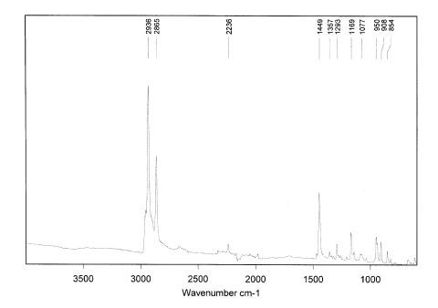
Figure B6.6 The IR spectrum for the ACCN ligand.
