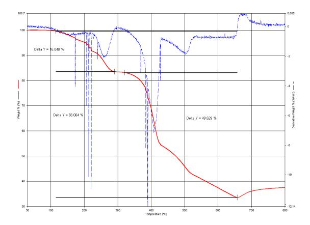
Figure 5.14 TGA (red) and DTA (blue) profiles for 5b. The very sharp blue lines of derivative DTA due to the possible moving of sample during heating and should be ignored.
