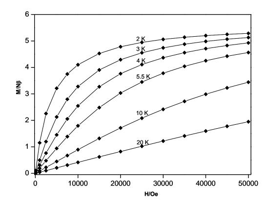
**Figure 3.20** The DC magnetization isotherms (0-5 T) for **3b**, per [Mn<sup>II</sup>Fe<sup>II</sup>].
