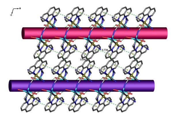
**Figure 3.12** 2-D sheet generated through a combination of self-complementary  $O-H\cdots O$  hydrogen bonds and  $\pi-\pi$  interactions. The red and purple cylinders indicate the way to produce pseudo 1-D tubes.
