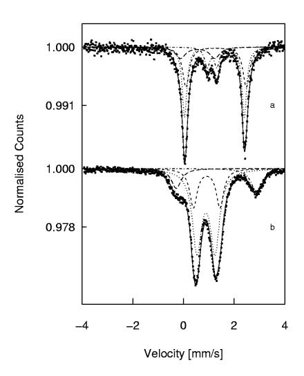
**Figure 6.14** <sup>57</sup>Fe Mössbauer spectra of [Fe<sup>II</sup>(AIBN)<sub>3</sub>][In<sup>III</sup>Cl<sub>4</sub>]<sub>2</sub> (**6a**) recorded at (a) 77 and (b) 295 K.
