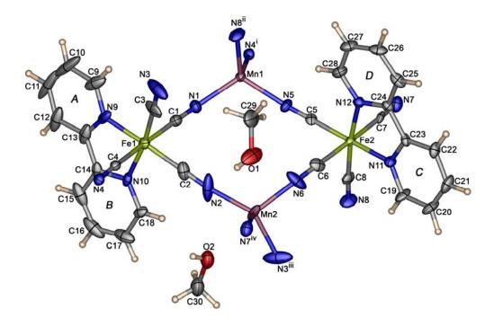
**Figure 3.1** Thermal ellipsoid plot of a fragment at the 50% probability level containing the asymmetric unit with atom numbering and showing coordination environments of metals centre in **3a**. Hydrogen atoms are shown as small spheres of arbitrary radii. The labeling scheme, A-D, applied to the phenyl rings is used to identify the rings in subsequent discussion. Symmetry codes: (i) -1+x, y, z; (ii) x, 0.5-y, -0.5+z; (iv) 1+x, y, z.
