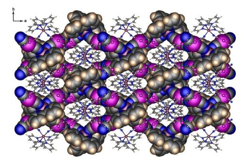
**Figure 4.4** Crystal packing in **4a** along the *c* axis showing a single (space-filling) and second (ball and stick) square grids formed *via* Ag···N, C–H··· $\pi$  and  $\pi$ ··· $\pi$  interactions.
