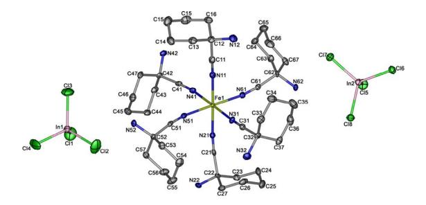
Figure 6.9 A view showing asymmetric unit with the atom numbering in 6c. Thermal ellipsoids are drawn at the 50% probability level at 123 K. The hydrogen atoms are omitted by simplicity. 6d is isostructural.
