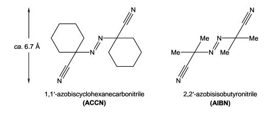
Scheme 1 The ligands (left) ACCN and (right) AIBN used for this study. They are capable of binding to two metal ions *via* the C≡N nitrogen donors but not *via* the azo group.
