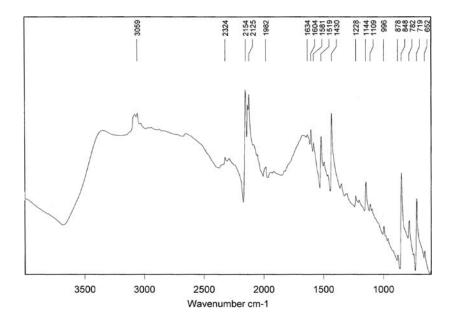
**Figure B3.5** The IR spectrum for  $H[Fe^{III}(1,10\text{-phen})(CN)_4] \cdot 2H_2O$ .
