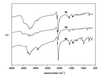
Figure B3.2 The IR spectrum for 3c-3e.
