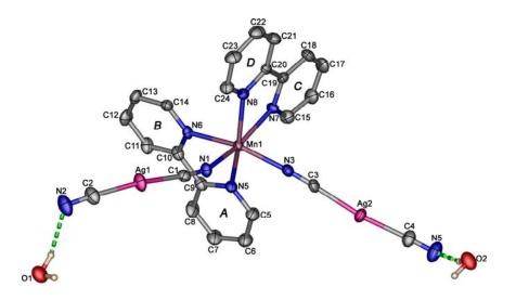
Figure 4.1 Perspective view of 4a with the atom-numbering scheme. Displacement ellipsoids are drawn at the 50% probability level. Hydrogen atoms are shown as small spheres of arbitrary radii. The labeling scheme, A-D, applied to the phenyl rings are used to identify the rings in subsequent discussion.
