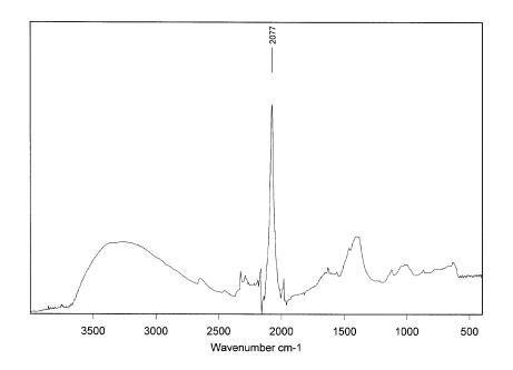
Figure B3.6 The IR spectrum for KCN.
