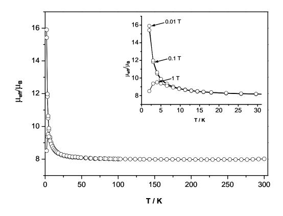
Figure 3.17 Plot of magnetic moment, per 2[Mn<sup>II</sup>Fe<sup>II</sup>], in fields of 0.01, 0.1 and 1 T for 3a. The 2–30 K region is expanded in the insert. The solid lines are not calculated plots.
