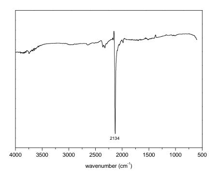
Figure B4.5 The IR spectrum for K[Ag(CN)<sub>2</sub>].
