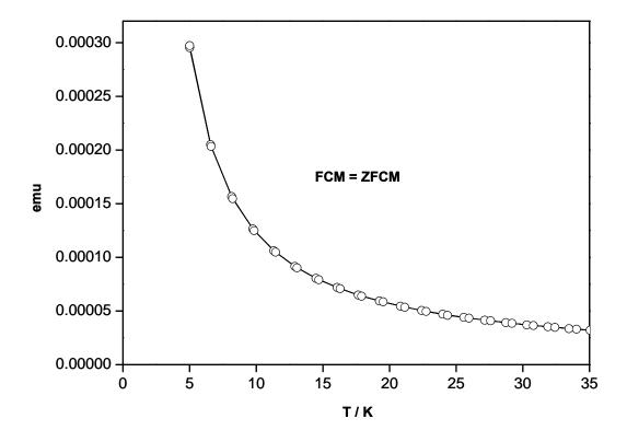
**Figure 3.21** Temperature dependence (4–35 K) of FCM and ZFCM for **3b**, in emu units from the SQUID instrument.
