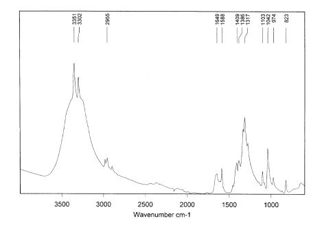
Figure B3.7 The IR spectrum for  $[Ni(en)(H_2O)_4](NO_3)_2$ .
