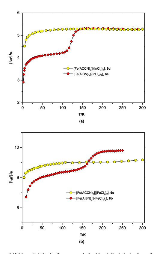
Figure 6.13 Magnetic behavior for compounds 6a–6d and 6b–6e in the form of  $\mu_{eff}$  vs *T* plots.
