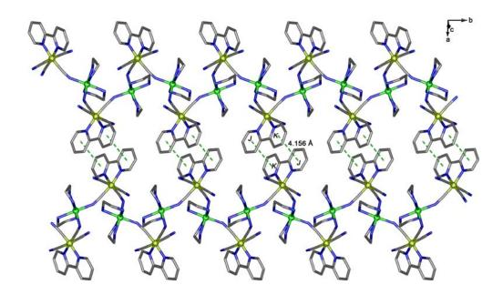
**Figure 3.15** View of the 1-D zigzag chains in **3e** running parallel to the *b* axis. Intermolecular  $\pi$ - $\pi$  contacts represented by dotted green lines are observed between the 2,2'-bipy ligands of adjacent chains.
