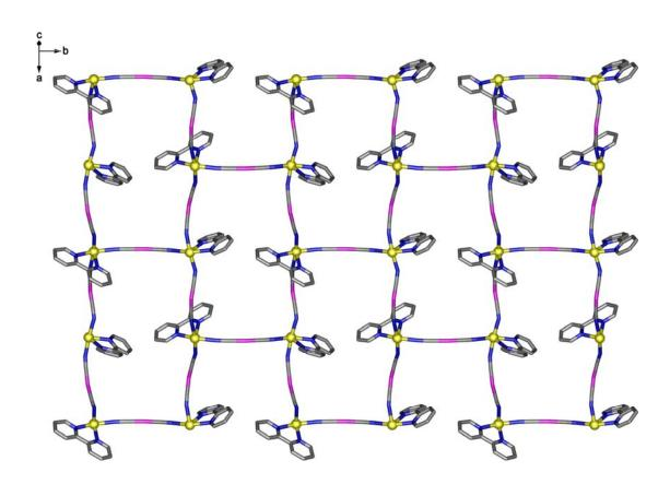
Figure 4.15 The 2-D sheet with the (6,3) topology in 4c.
