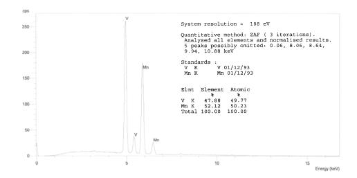
Figure B7.4 The EDX spectrum for 7b.
