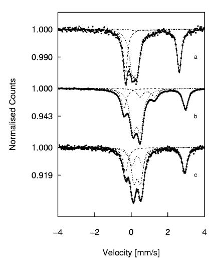
Figure 6.15 <sup>57</sup>Fe Mössbauer spectra of  $[Fe^{II}(AIBN)_3][Fe^{III}Cl_4]_2$  (6b) recorded at (a) 4.2, (b) 77, and (c) 295 K.
