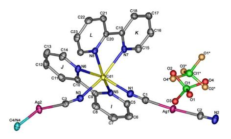
Figure 4.9 Perspective view of 4c with the atom-numbering scheme. Displacement ellipsoids are drawn at the 50% probability level. Hydrogen atoms are omitted for clarify. The labeling scheme, *I-L*, applied to the phenyl rings are used to identify the rings in the subsequent discussion.
