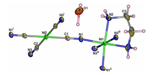
Figure 5.1 View of 5a with the atom-numbering scheme. Displacement ellipsoids are draw at the 50% probability level. Hydrogen atoms are shown as small spheres of arbitrary radii. Symmetry codes: (i) 0.5-x, 0.5-y, 1-z; (ii) -x, y, 0.5-z; (iii) 0.5+x, 0.5+y, z; (iv) 0.5-x, 0.5+y, 0.5-z; (v) -x, y, 0.5-z.
