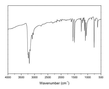
Figure B2.6 The IR spectrum for 2e.
