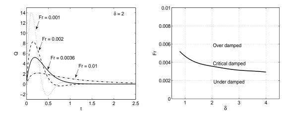
**Figure 5.5** Predicted variation of volume rate with time.
