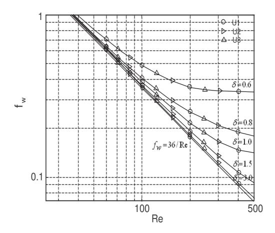
Figure 5.2 Friction factor as a function of Reynolds number.
