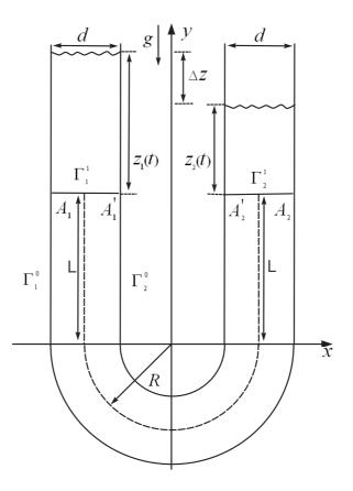
Figure 5.4 Schematic diagram of oscillating flow in U-bend channel.
