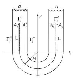
Figure 5.1 Schematic diagram of U-bend channel.
