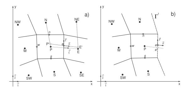
Figure 3.1 A typical 2D control volume with the notation used and a way of calculating cell face value and gradients.
