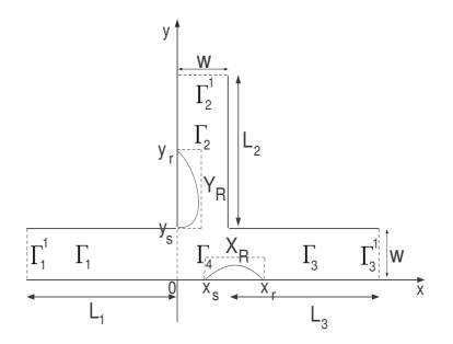
Figure 4.1 Schematic geometry of T-junction bifurcation and coordinate system.
