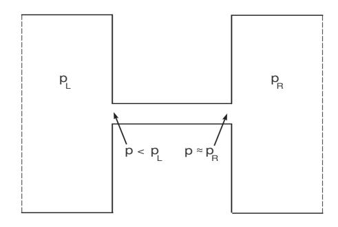
Figure 2.2 Flow in a pipe joining two plenums at different pressures.
