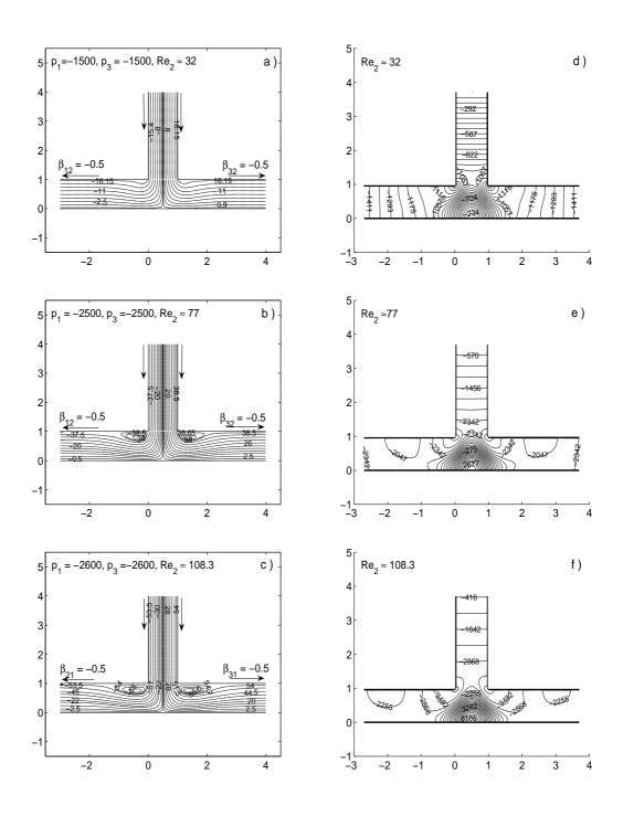
**Figure 4.8** The streamline (left column) and pressure contours (right column) for impacting T-junction. See cross signs  $(\times)$  on line *OG* in Figure 4.7.
