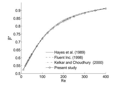
**Figure 4.2** The flow rate ratio,  $\beta^*$ , as a function of Reynolds number, *Re*.
