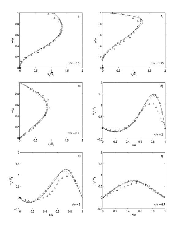
Figure 4.5 Comparison between experimental data of Liepsch *et al.* (1982) and numerical data of Miranda *et al.* (2008) ( $Re_Q = 248$  and  $\beta = 0.44$ ).
