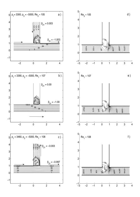
**Figure 4.11** The streamline (left column) and pressure contours (right column) for the case correspond to down triangle signs  $(\nabla)$  on line *OD* in Figure 4.7.
