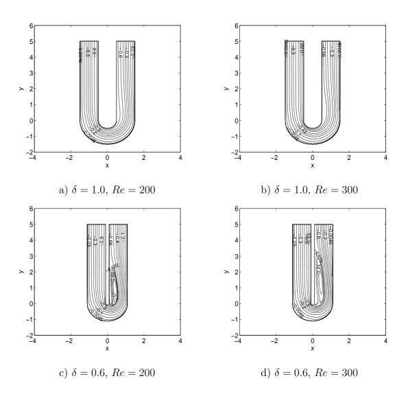
Figure 5.3 Streamline patterns of flow in the U-bend channel for various  $\delta$  and Re. technical devices. The study of frequency, amplitude, and damping factor cannot be done if velocity is given advanced on through-flow parts. By this end, we came to the boundary value problem with pressure given at through-flow parts. The flow configuration, the coordinate system, and the main notations are shown in Figure 5.4
