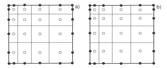
**Figure 1.1** Types of Finite volume grids, nodes centered in control volume (left), and control volume faces centered between nodes (right).
