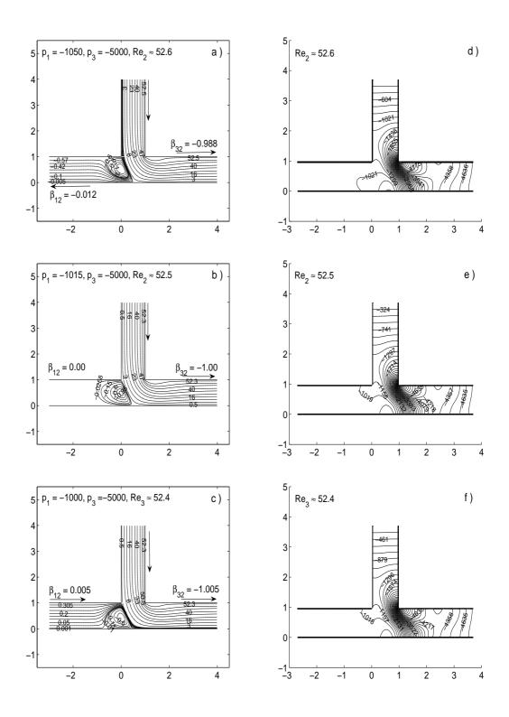
**Figure 4.10** The streamline (left column) and pressure contours (right column) for the case correspond to square signs ( $\Box$ ) on line *OF* in Figure 4.7.
