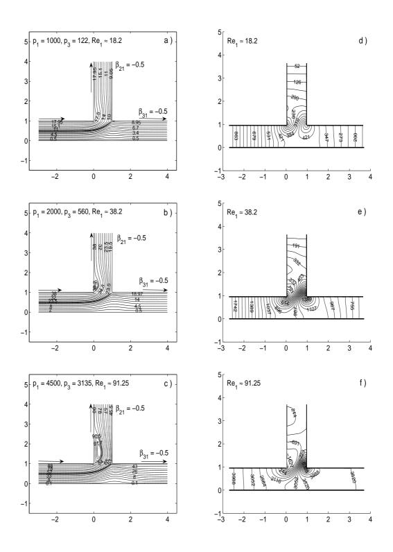
**Figure 4.9** The streamline (left column) and pressure contours (right column) for the case correspond to triangle signs ( $\triangle$ ) on line *OC* in Figure 4.7.
