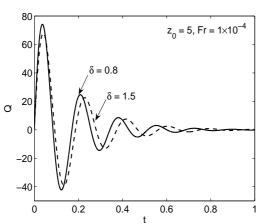
Figure 5.9 Variation of volume rate with time. Influence of curvature ratio  $\delta$ .
