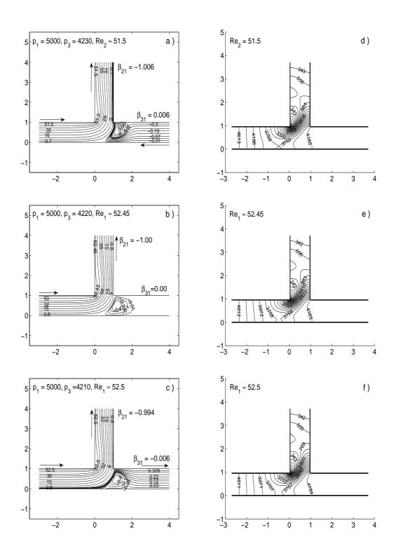
**Figure 4.12** The streamline (left column) and pressure contours (right column) for the case correspond to circle signs  $(\bigcirc)$  on line *OB* in Figure 4.7.
