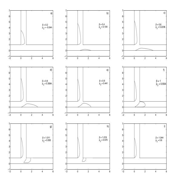
Figure 4.6 Developing of Main and secondary recirculation zone as a function of flow split  $\beta$ .
