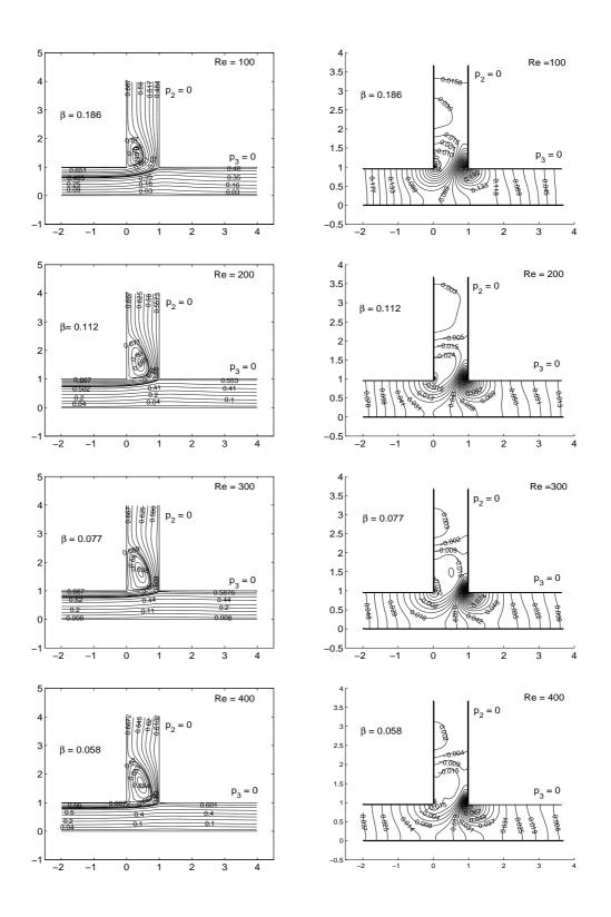
Figure 4.3 Streamline patterns and pressure contour of flow in the T-junction for various Re, and equal static pressure at the exists  $\Gamma_2^1$  and  $\Gamma_3^1$ .
