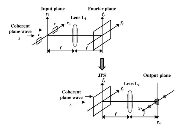
Figure 2.1 Schematic diagram for implementing joint transform correlation.
