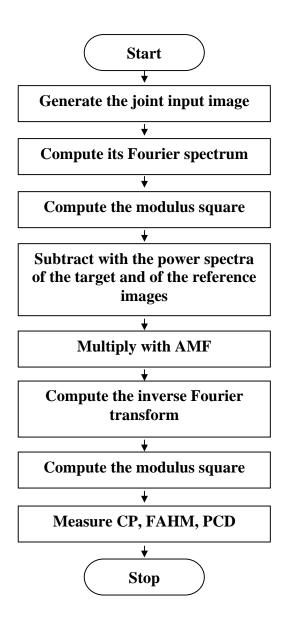
Figure 3.2 Flowchart for simulating the operation of the modified AMJTC.
