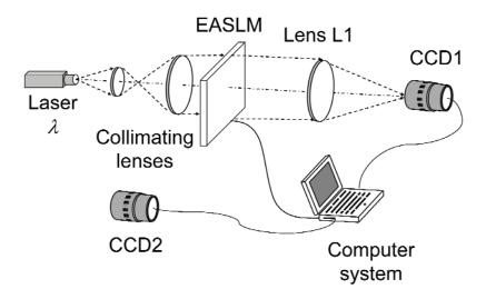
Figure 2.2 Schematic diagram of optical setup for implementing the real-time modified AMJTC.
