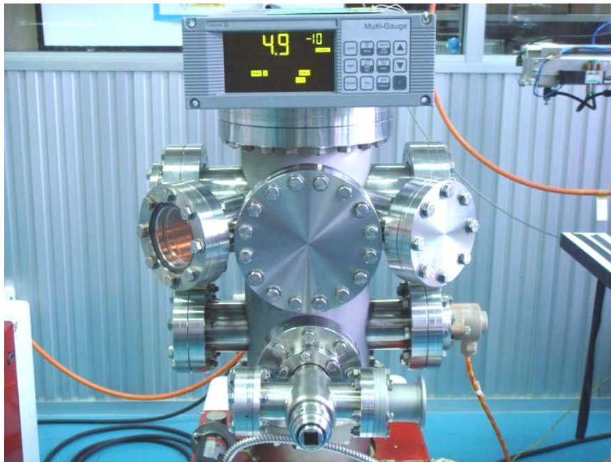
Figure 2.4 Demonstration of UHV level in the first vacuum chamber
