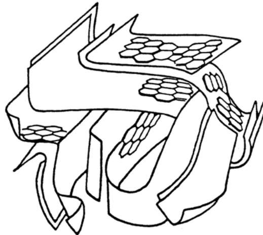
Figure 2.3 A schematic representation of the structure of activated carbon (Bansal, Donnet, and Stoeckli, 1988).
