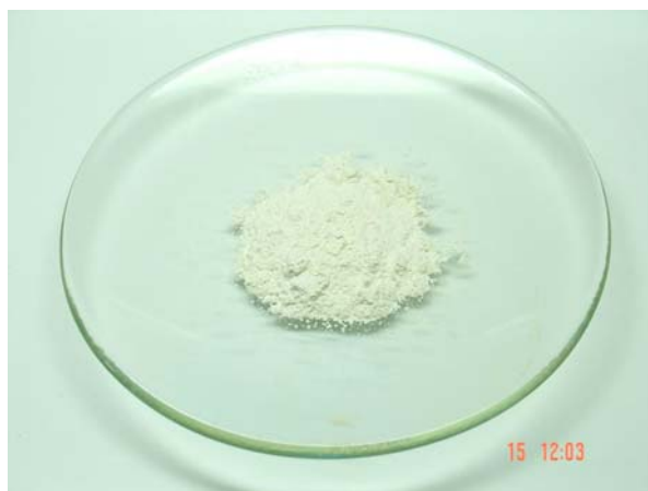
Figure 4.25 diatomite treated with hot 6M H 2 SO 4 for starting material
