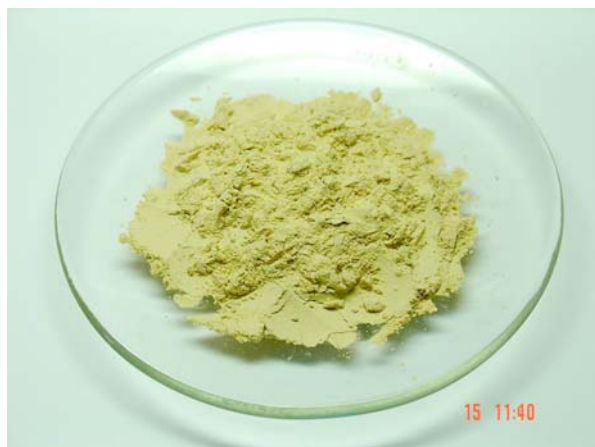
Figure 4.21 diatomite starting material
