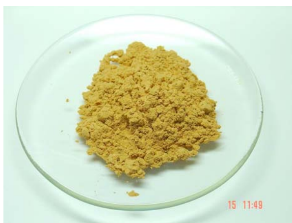
Figure 4.22 diatomite calcined at 900 °C for starting material
