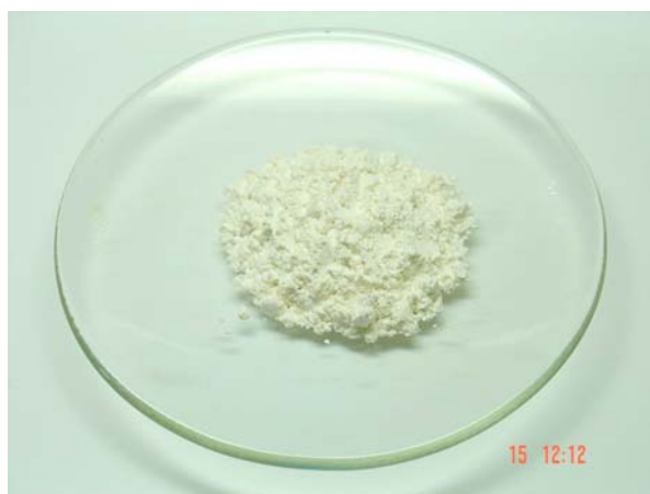
Figure 4.26 diatomite first treated with hot 6M H 2 SO 4 then calcined at 1100 °C for starting material
