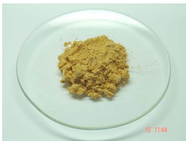
Figure 4.22 diatomite calcined at 900 °C for starting material
