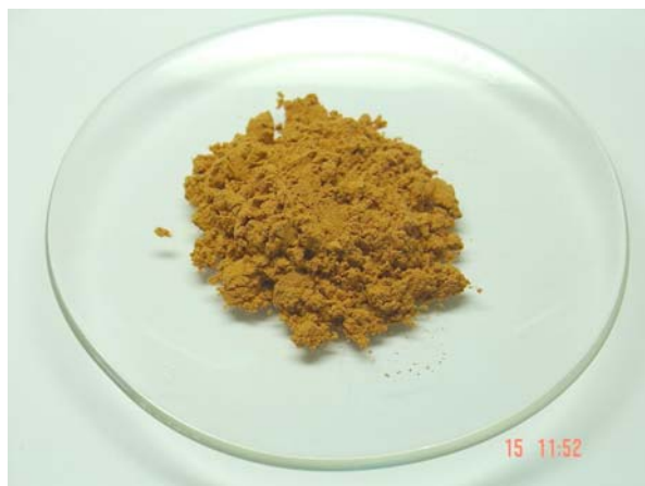
Figure 4.24 diatomite calcined at 1100 °C for starting material
