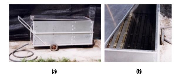
Fig 5 Photos of 540L fermentor that made from stainless steel (3 wheels drive), comportable for movement, there are tube and its connection line for stearning a Front view, b. Inside Fermentor have sieve to contain substrate during sterile and fermentation
