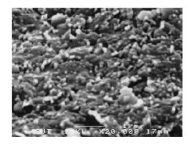
Figure 3.3 SEM picture of silica surfaced with magnification of 10 kV x 20,000
