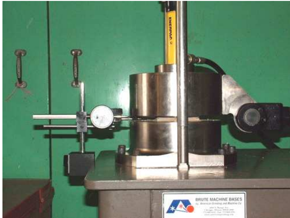
Figure 4.2 Test arrangement of saw-cut surface specimen used in the direct shear test with direct shear machine model SBEL DR440.
