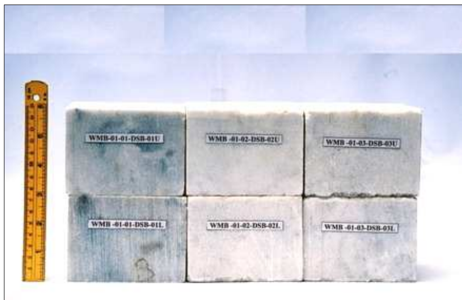
Figure 3.11 Saw-cut surface specimens of marble prepared for direct shear test with block size 10 \times 10 \times 7.5 cm.
