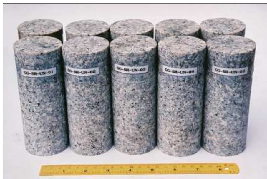
Figure 3.7 Granite specimens prepared for uniaxial compressive strength testing with 54 mm diameter and L/D ratio equal to 2.5.
