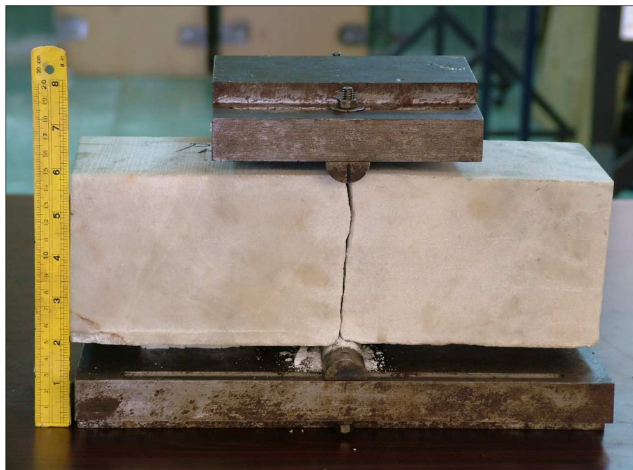
Figure 3.13 Splitting tensile fractures of marble specimens prepared for direct shear testing.
