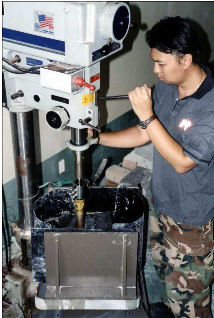
Figure 3.3 Drilling machine (model SBEL 1150) is used to drill core specimens with 54 mm diameter.
