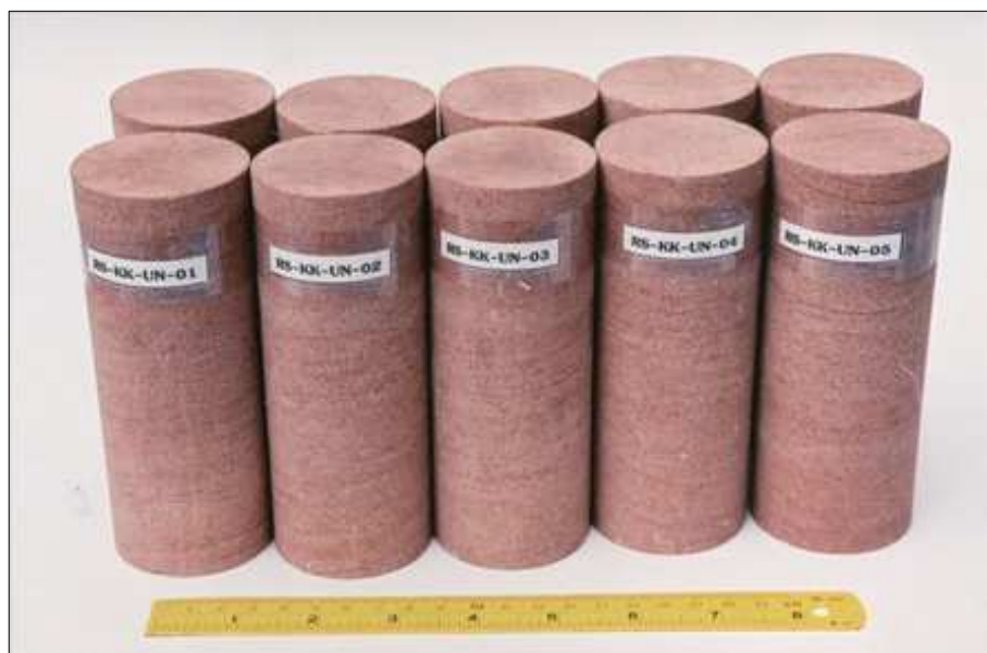
Figure 3.9 Sandstone specimens prepared for uniaxial compressive strength testing with 54 mm diameter and L/D ratio equal to 2.5.
