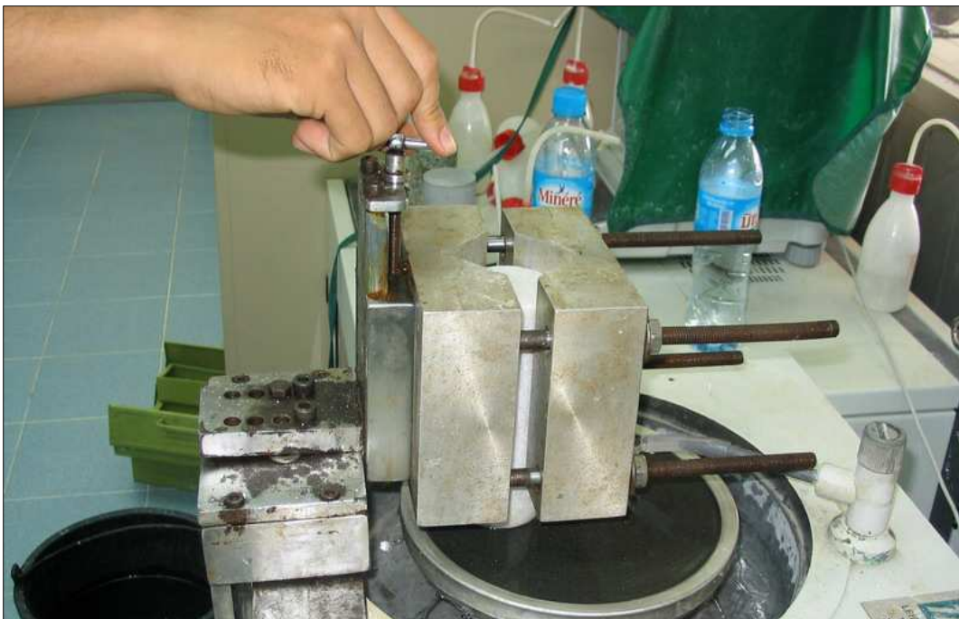
Figure 3.5 Grinding of core sample for smooth and parallel end surfaces.
