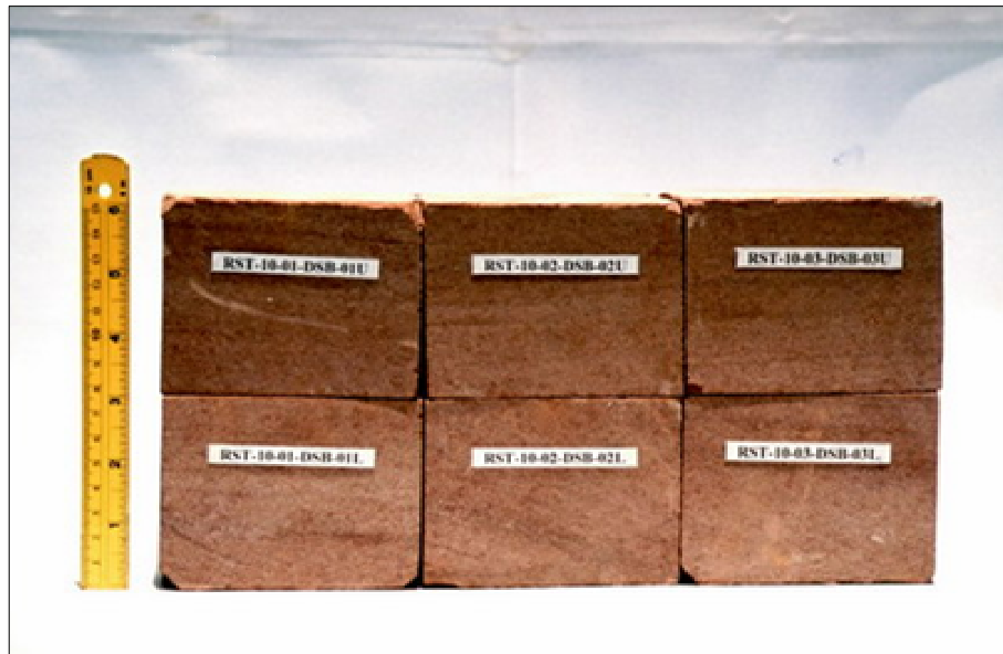
Figure 3.12 Saw-cut surface specimens of sandstone prepared for direct shear test with block size 10 \times 10 \times 7.5 cm.
