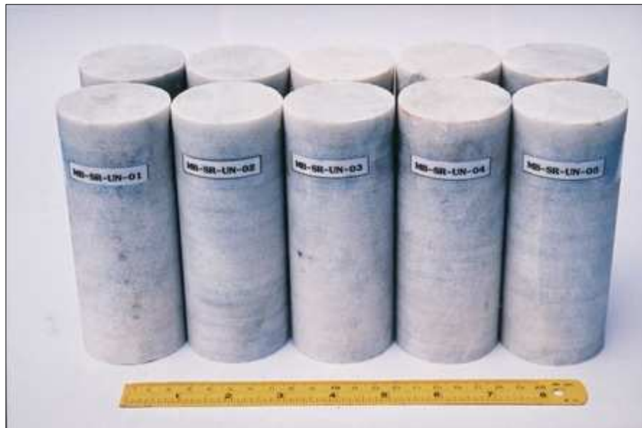
Figure 3.8 Marble specimens prepared for uniaxial compressive strength testing with 54 mm diameter and L/D ratio equal to 2.5.
