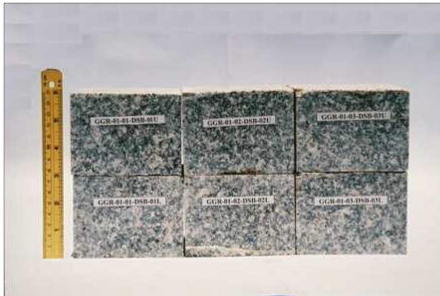
Figure 3.10 Saw-cut surface specimens of granite prepared for direct shear test with block size 10 \times 10 \times 7.5 cm.
