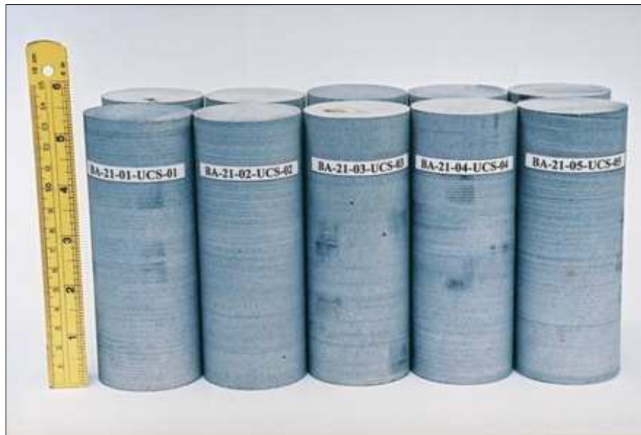
Figure 3.6 Basalt specimens prepared for uniaxial compressive strength testing with 54 mm diameter and L/D ratio equal to 2.5.
