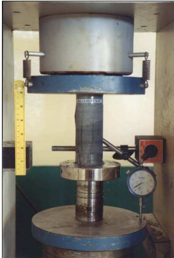
Figure 4.1 Uniaxial compressive strength test on 54 mm diameter specimen with L/D ratio equal to 2.5. The specimen is loaded axially in compression machine model ELE-ADR2000.
