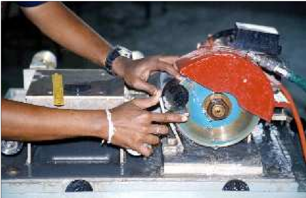
Figure 3.4 Core sample is cut to obtain the desired length.
