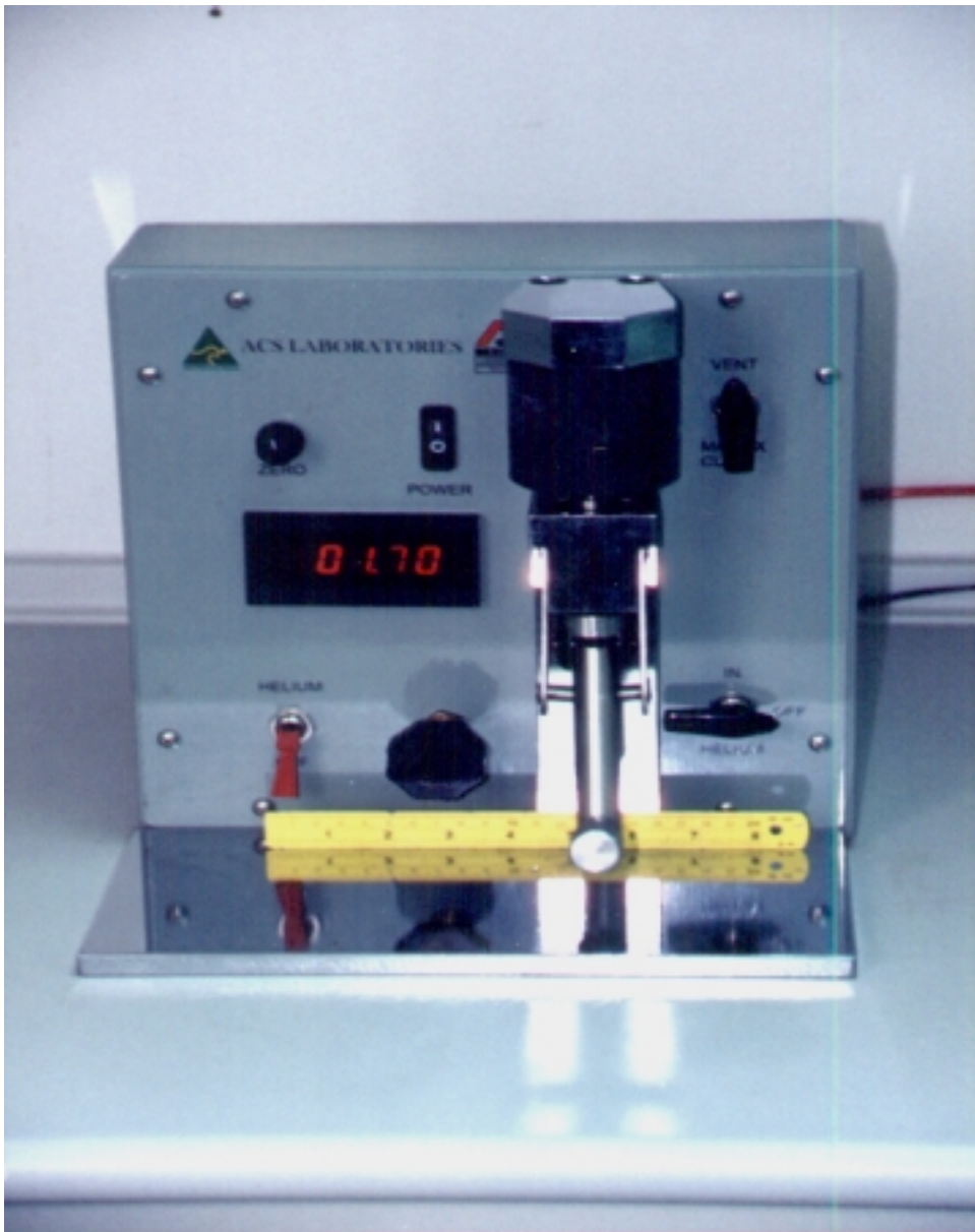
Figure 3.4 The porosimeter instrument is used for measuring the porosity of the specimens.
