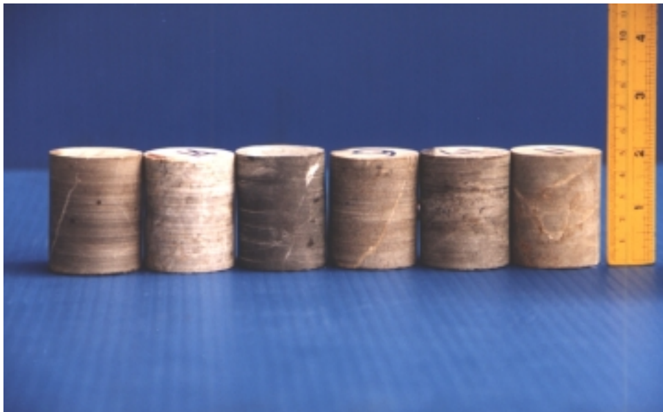
Figure 3.3 The specimen shape is cylinder. The specimen size is two inches in length and one and a half five inches in diameter.
