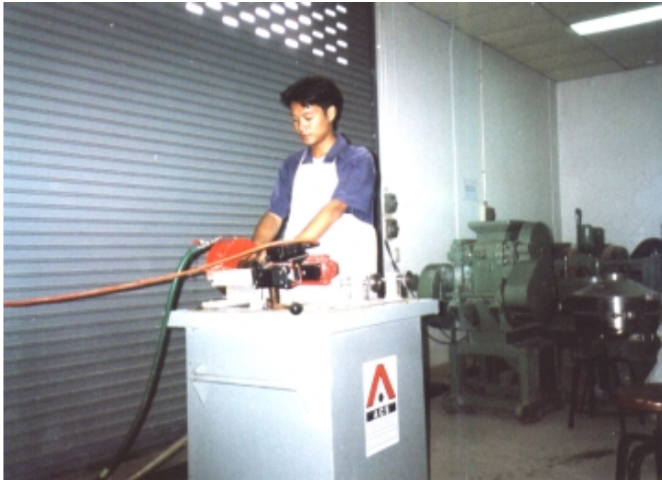
Figure 3.1 Coring Machine is the instrument that uses for drilling the rock samples with cylinder shape.
