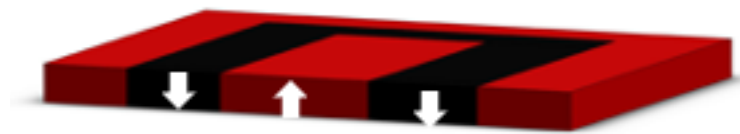
Figure 3.6 The phase image shows different polarization direction when voltage is applied to the sample surface.
