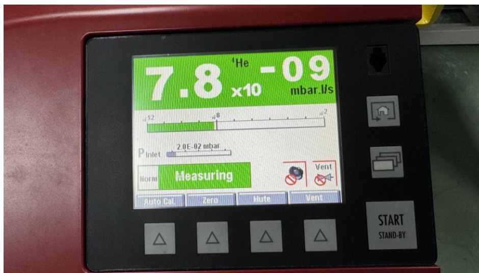
Figure 4.17 Digital display of the helium leak rate during vacuum component testing.
