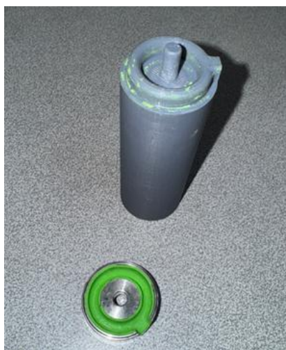
Figure 4.20 Pressing the tamper into modeling clay in the ionizer body's grooves, simulating the application of alumina paste ( \text{Al}_2\text{O}_3 ).
