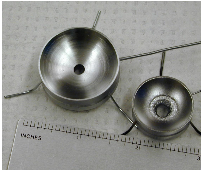
Figure 3.8 Comparison of a new ionizer (left) and a used ionizer (right), showing burn marks at the center caused by sputtered ions spreading in all directions and striking the surface Ref. Purdue University Prime Lab. (n.d.). Ionizer.
