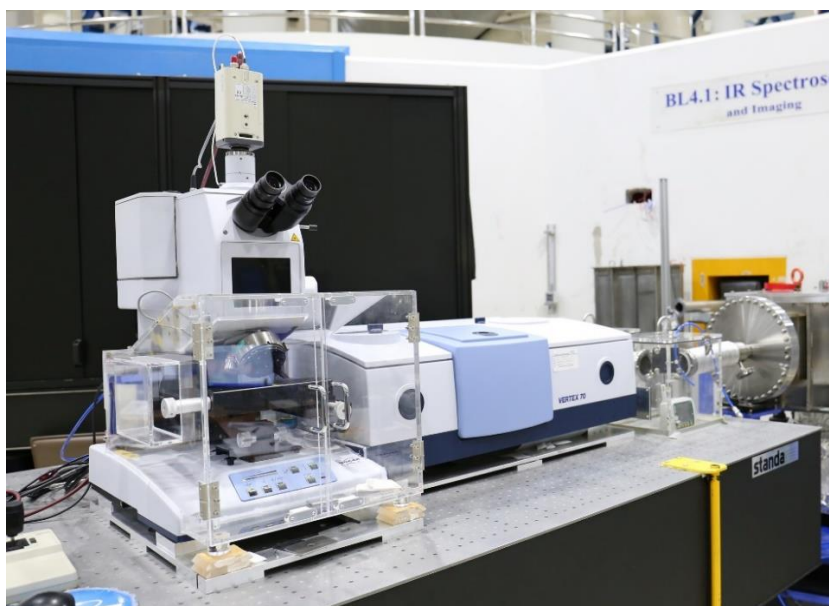
Figure 3.5 Bruker VEXTX 70 vacuum FTIR spectroscopy system linked to a Bruker Hyperion 2000 IR microscope (Bruker Optics, Ettlingen, Germany) at beamline 4.1 of the Synchrotron Light Research Institute (Public Organization), Thailand.
