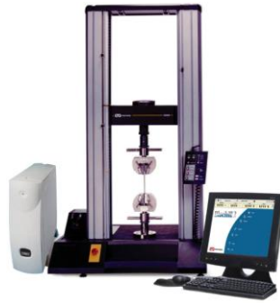
Figure 3.3 Universal testing machine (INSTRON/5565, Norwood, MA, USA).
