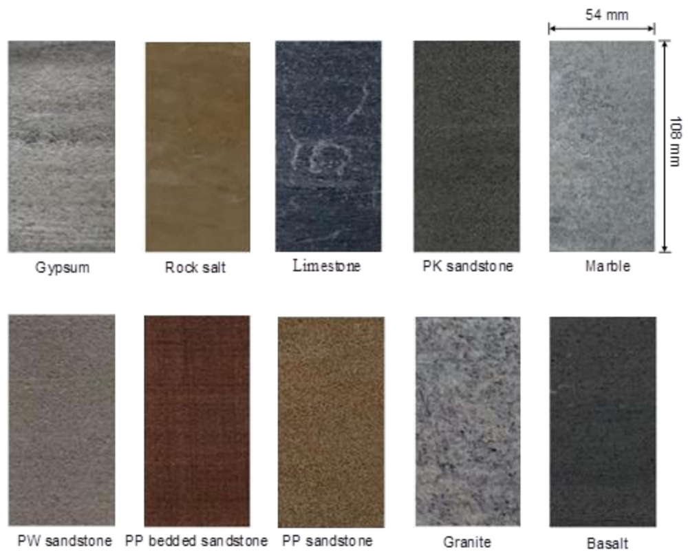
Figure 3.2 Some specimens prepared for single and multi-stage triaxial compression tests
