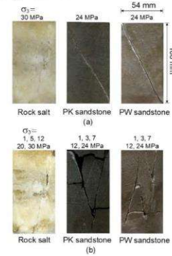
Fig.2. Some post-test specimens for single stage (a) and multi-stage triaxial compression tests (b).
