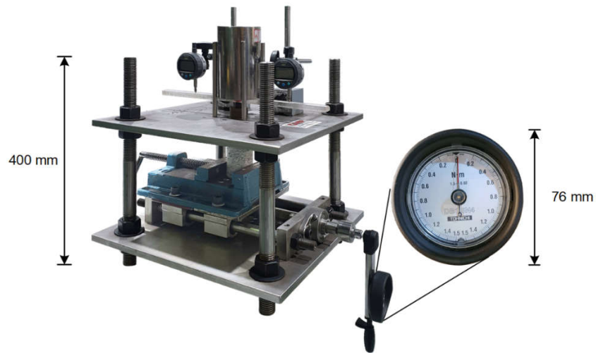
Figure 4.1 Device based on West CERCHAR apparatus with additional torque and vertical displacement measurements (Kathancharoen and Fuenkajorn, 2023).
