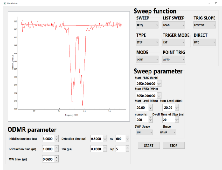
Figure 3.5 The Sweeping program is designed by Qt designer. The program has three main parts “Sweep function”, “Sweep parameter” and “ODMR parameter”.
