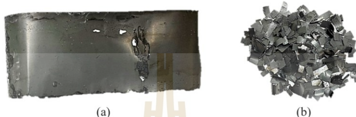
Fig. 1. Cathode material a) cathode b) reduced size of the cathode.
