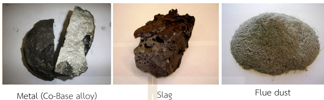
Figure 2.14 Products from battery smelting in an EAF furnace (left) metal, (center) slag, and (right) dust (Georgi-Maschler et al., 2012).
