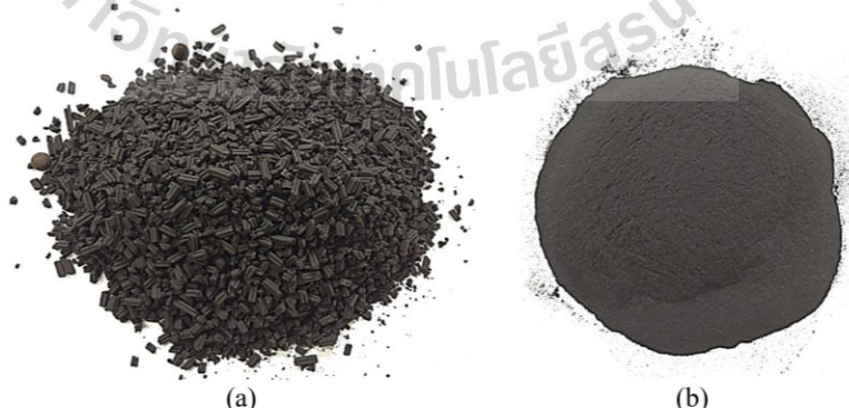
Fig. 2. Ni-Mo spent catalyst (a) as received, (b) crushed sample.
