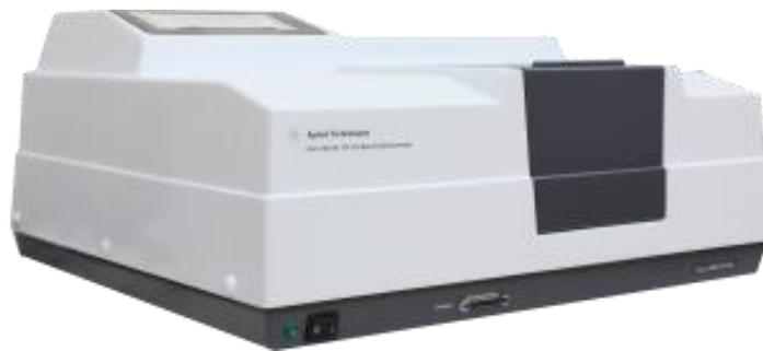
**Figure 3.15** UV-vis spectrophotometer at SUT (<http://cste.sut.ac.th/2014/?p=945>).
