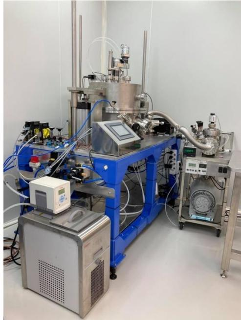
**Figure 3.4** RF magnetron sputtering system at BL6, SLRI.
