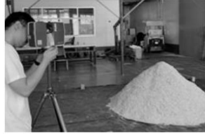
Fig. 3 Verified for accuracy using a FARO focus.
