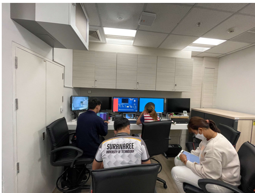
Figure 4.14 The control room has monitors for requiring users to adjust patient bed position, parameterise proton beam and creating treatment plan.
