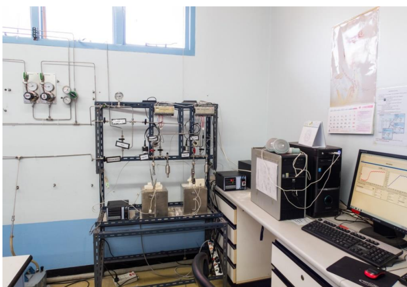
Figure 3.8 Laboratory-scale setup of Sievert-type apparatus.
