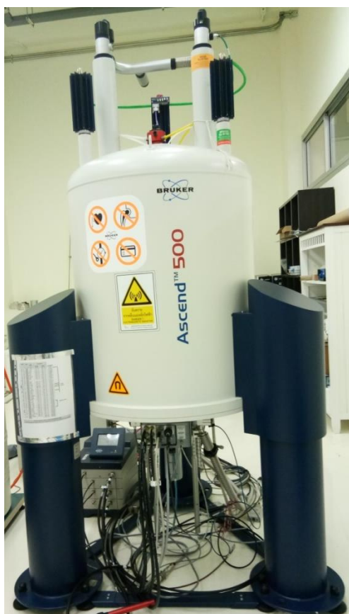
Figure 3.5 A Bruker Ascend TM 500 Solid-State magic-angle spinning nuclear magnetic resonance (MAS NMR) spectrometer (A) and zirconia end-capped tube (B).
