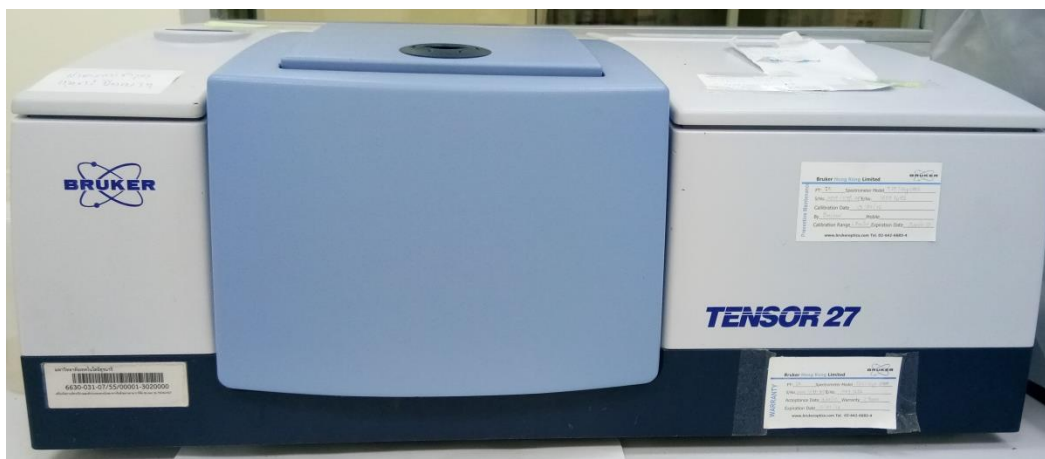
Figure 3.3 A Bruker Tensor 27 Fourier transform infrared spectrophotometer.
