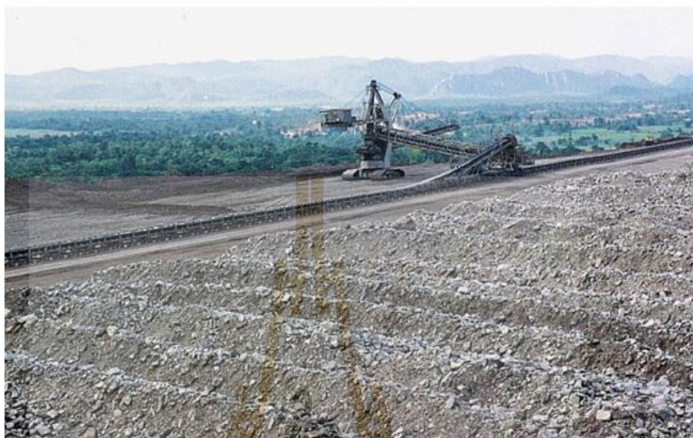
Fig. 2. Spreading the waste dump materials to the dumping area via a conveyor system.
