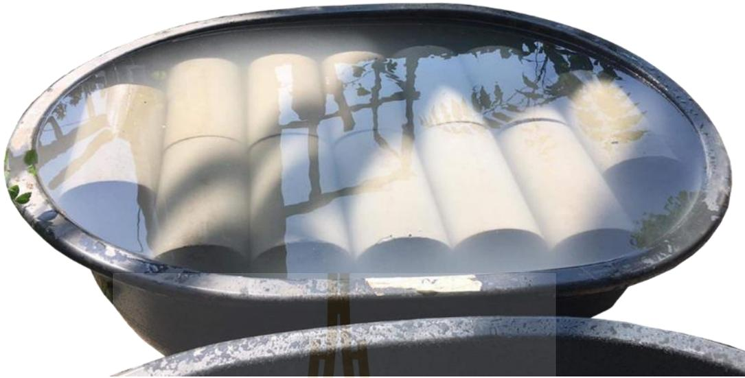
Figure 3.11 The concrete samples were submerged in tap water for a curing period of up to 28 days.
