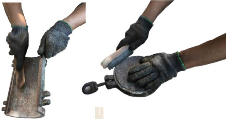
Figure 3.5 Preparing the concrete molds involved scrubbing them with a wire brush and applying oil to the formwork, facilitating the easier removal of the concrete samples from the molds.
