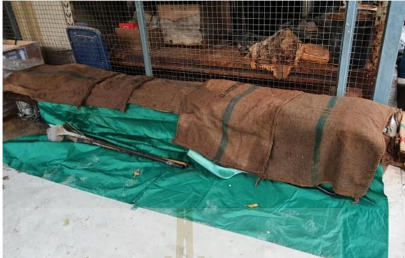
Figure 3.9 After casting, the samples are covered with a hemp sack and left to set before being removed from the mold.
