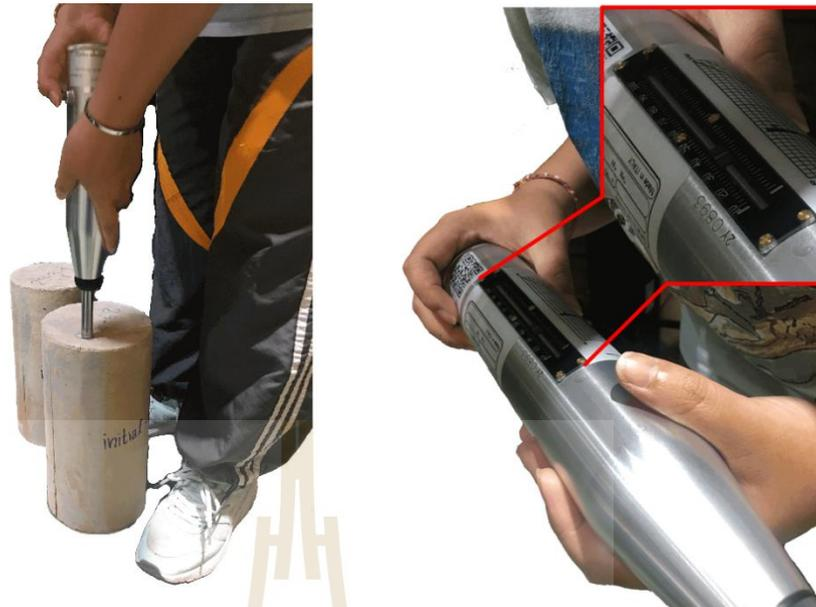
Figure 4.2 Schmidt rebound hammer testing of a concrete sample.
