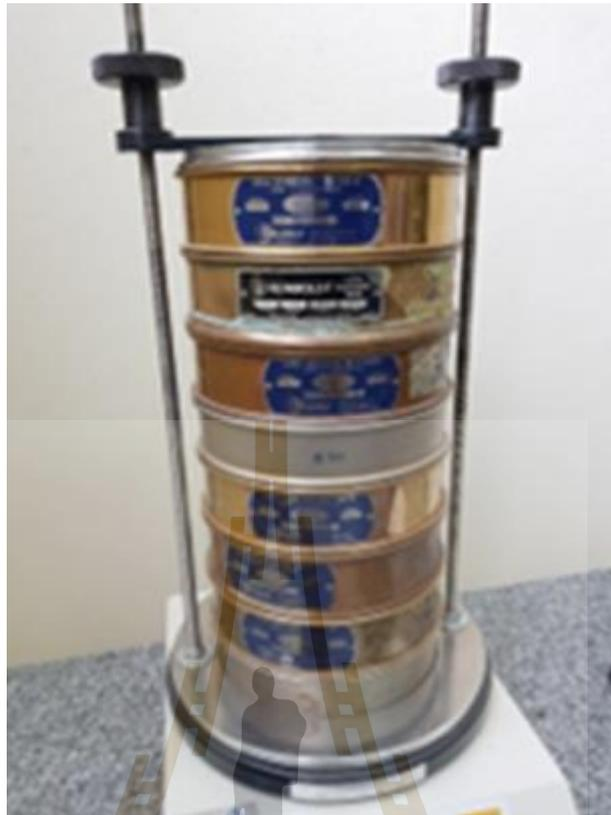
Figure 3.3 Analysis of the particle sizes in both the fine and coarse aggregates was conducted using a vibrator and sieve method in accordance with ASTM C136 standards. This analysis was performed before the aggregates were mixed with cement and water.
