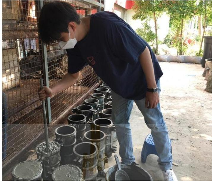
Figure 3.7 Steel rods are used to prod the liquid concrete, eliminating air bubbles, and ensuring complete filling within the mold.
