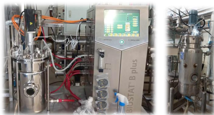
Figure 2.15 5 L fermentor and 50 L fermentor systems.
