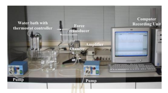
Figure 4.1 Representation of equipment used for tension measurement.
