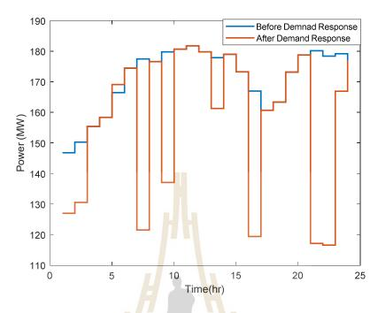
Figure 4.23 Comparison of load pattern before and after demand response in Case II
