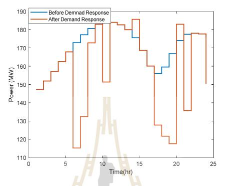
Figure 4.25 Comparison of load pattern before and after demand response in Case IV
