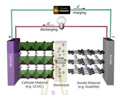
Figure 2.1 A schematic diagram of a typical LIB (Liu et al., 2011).
