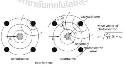
Figure 2.12 Interference of outgoing and backscattered photoelectron wave.
