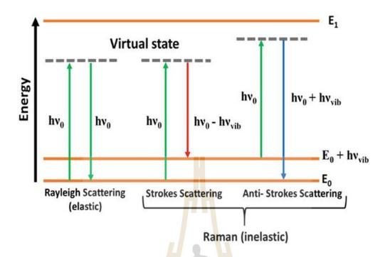
Figure 2.16 Basics principle of state diagram of scattering pattern.
