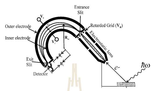
Figure 2.14 A schematic diagram of typical XPS experiment.
