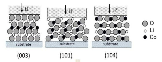
Figure 2.7 Schematic diagram showing the preferred textures for sputtered LiCoO<sub>2</sub> films.
