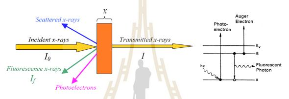
Figure 2.7 Schematic of incident and transmitted X-ray beam.
