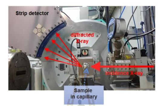
Figure 3.1 A photograph of powder X-ray diffraction (PXRD) end-station of BL1.1W, SLRI.
