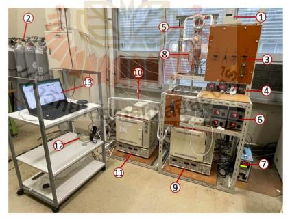
**Figure 5.1** AASR setup: (1) Feed injector: flow acetic acid solution into the flow reactor, (2) Gas tank, (3) Gas value: open and close gas from tank, (4) Flow meter: setting gas flow rate, (5) Gas line<sub>(in)</sub>: flowing  $N_2$  as carrier gas into flow reactor, (6) Heater: heating
