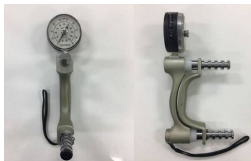
Figure 3.7 JAMAR hand dynamometer as a measuring tool for grip strength measurement.
