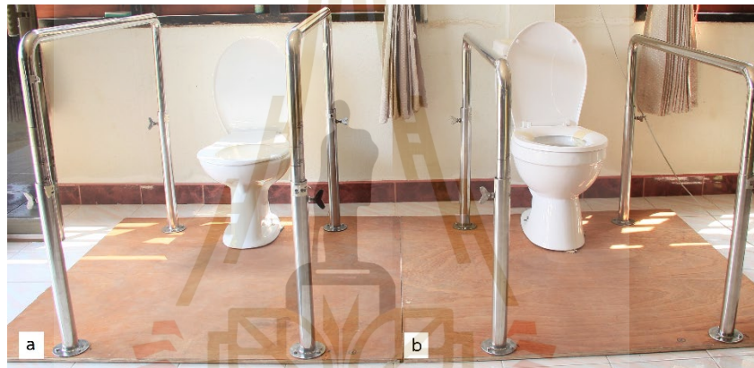
Figure 3.5 Stand-to-sit and sit-to-stand time measurement experimental set up with adjustable handrail height: (a) conventional toilet and (b) modern toilet.
