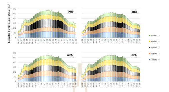
Figure 4.9 Estimated Traffic Volume of Different Road Sections
