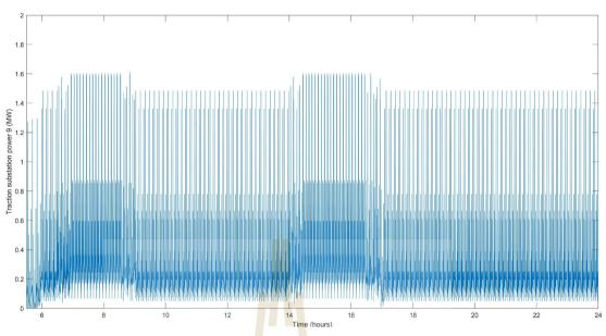
Figure A. 17 Wongsawang traction substation load curve
