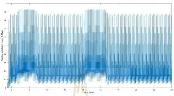
Figure A. 13 Nonthaburi Center traction substation load curve
