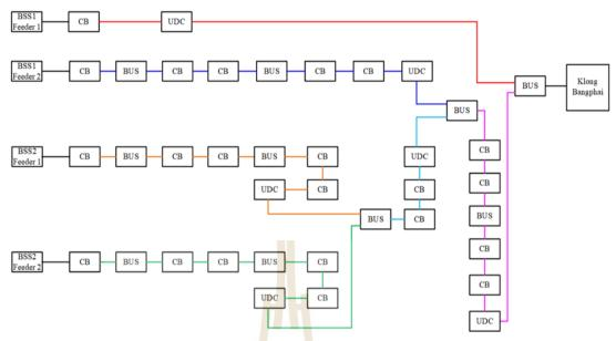
Figure 3. 19 Klong Bangphai substation block combination
