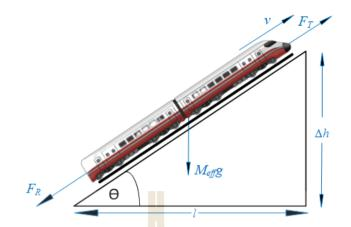
Figure 2. 8 Free body diagram of the train movement
