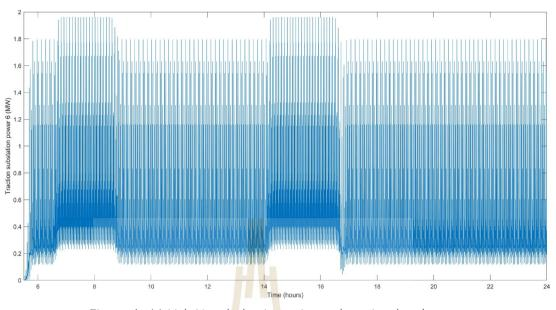
Figure A. 11 Yak Nonthaburi traction substation load curve
