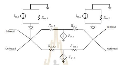
Figure 2. 11 The equivalent circuit of DC railway power supply systems
