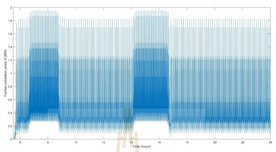
Figure A. 9 Saima traction substation load curve
