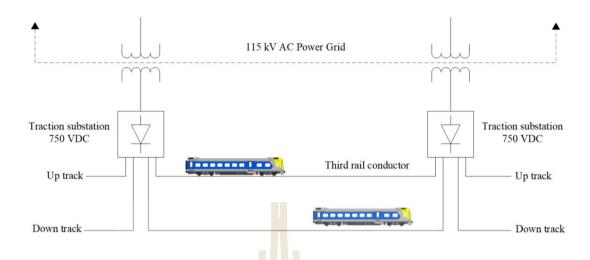
Figure 2. 7 Circuit diagram of a typical DC railway power system
