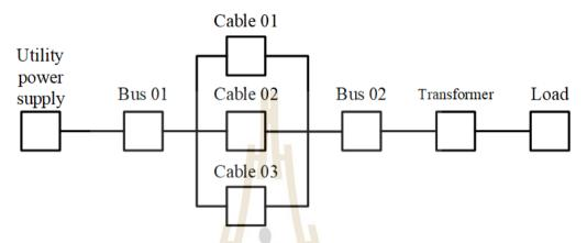
Figure D. 1 Simple circuit block for calculation in ETAP
