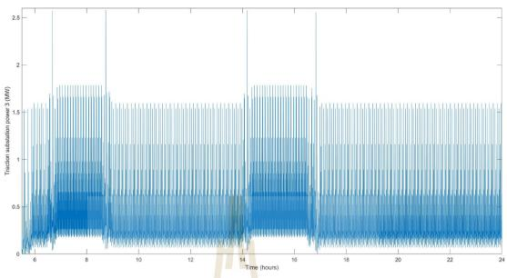
Figure A. 5 Bangyai traction substation load curve
