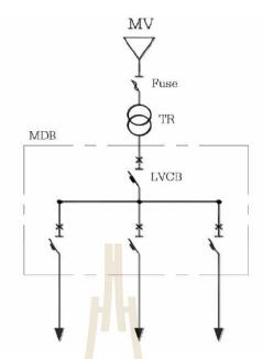
Figure 2. 12 Radial system circuit
