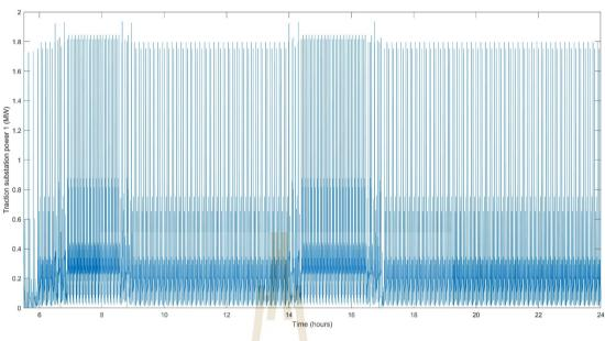
Figure A. 1 Klong Bangphai traction substation load curve
