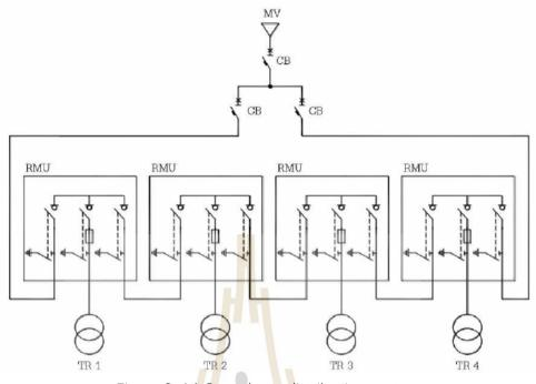
Figure 2. 16 Open-loop distribution system
