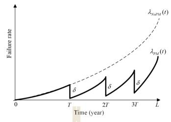
Figure 2. 6 Preventive maintenance model for failure rate.
