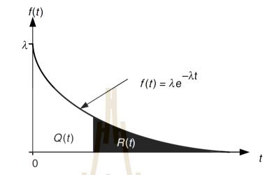
Figure 2. 1 Exponential density function and R(t) and Q(t)
