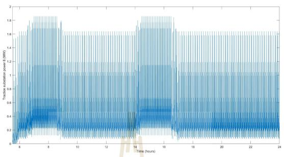
Figure A. 15 Yak Tiwanon traction substation load curve
