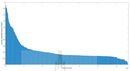
Figure 3. 7 Saima traction substation load duration curve
