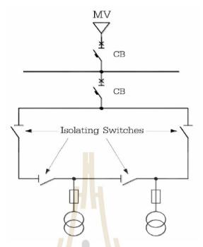
Figure 2. 15 Closed-loop distribution systems circuit
