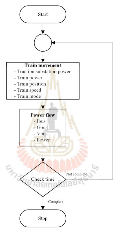
Figure 3. 2 The procedure for calculating multi-train simulation
