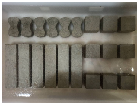
Figure 3.2 Curing of the test specimens.
