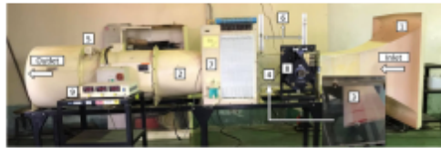
Fig. 4. PLINT TE54/8418 subsonic wind tunnel and its accessories.
