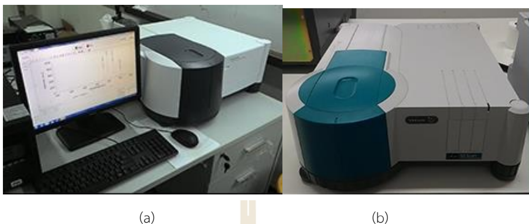
Figure 3.6 (a) Fluorescence Spectrophotometer (Cary-Eclipse)(Photo-luminescence measurement of material in visible region from 200 - 900 nm) and (b) UV-VIS spectrophotometer (Cary-50) (and %T measurements in the range of 200 - 1100 nm with CIE L*a*b*color coordinate software).
