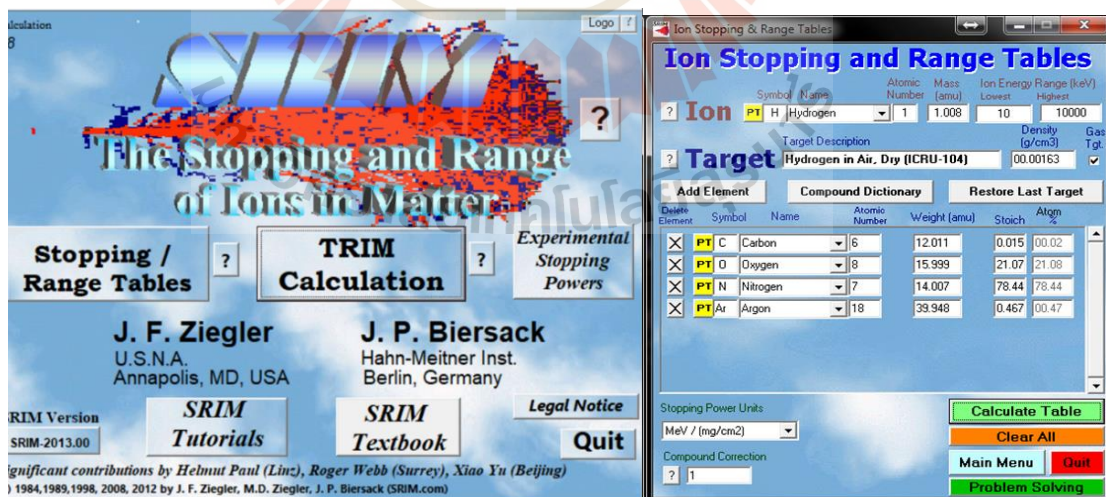
Figure 2.22 SRIM window of input parameters for stopping calculation.
