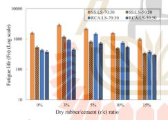
Fig. 8. ITFL of cement- and cement-NRL stabilized SS:LS and RCA:LS blends at different SS/RCA replacements and r/c ratios.
