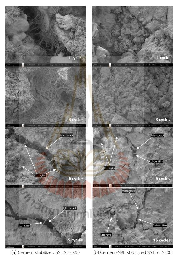
Figure 5.10 SEM images of cement-NRL stabilized SS:LS=70:30 at (a) r/c ratio = 0% and (b) r/c ratio = 3% at 1<sup>st</sup>, 3<sup>rd</sup>, 6<sup>th</sup>, and 15<sup>th</sup> cycles.
