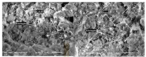
(a) SS:LS=70:30 at r/c ratio of 0% (b) RCA:LS=70:30 at r/c ratio of 0%
