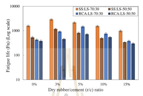
**Figure 4.8** Fatigue life (Fn) of cement- and cement-NRL stabilized SS:LS and RCA:LS blends at different SS/RCA replacements and r/c ratios.
