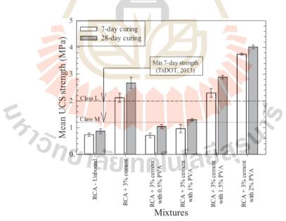
Figure 2.12 UCS values of cement stabilized RCA and cement-PVA stabilized RCA at 7day and 28-day cured times (Yaowarat et al., 2020)
