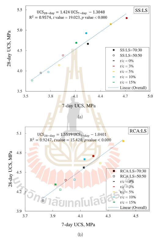
Figure 3.9 Relationship between 7-day and 28-day UCS of cement-NRL stabilized (a) SS:LS and (b) RCA:LS samples at different r/c ratios.
