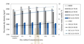
Fig. 2. The illustration of compaction characteristics of mixtures.
