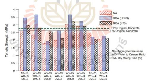
**Figure 2.9** Splitting tensile strength of RCA and NA concretes with varied conditions of aggregate size, w/c ratio, and dry mix time (Tavakoli & Soroushian, 1996)
