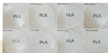
Figure 4. Photographs of films prepared from PLA and PLAnanocomposites (250-300 μm thickness)
