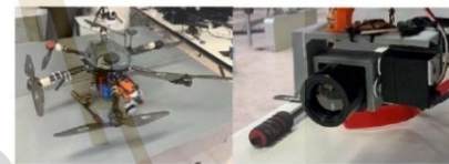
Fig. 3. UAV's thermal camera.
