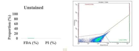
Figure 4.6 Flow cytometric analysis with permeable esterase substrate fluorescein diacetate (FDA) and the cell impermeable DNA stain propidium iodide (PI). Unstained cell used for control.
