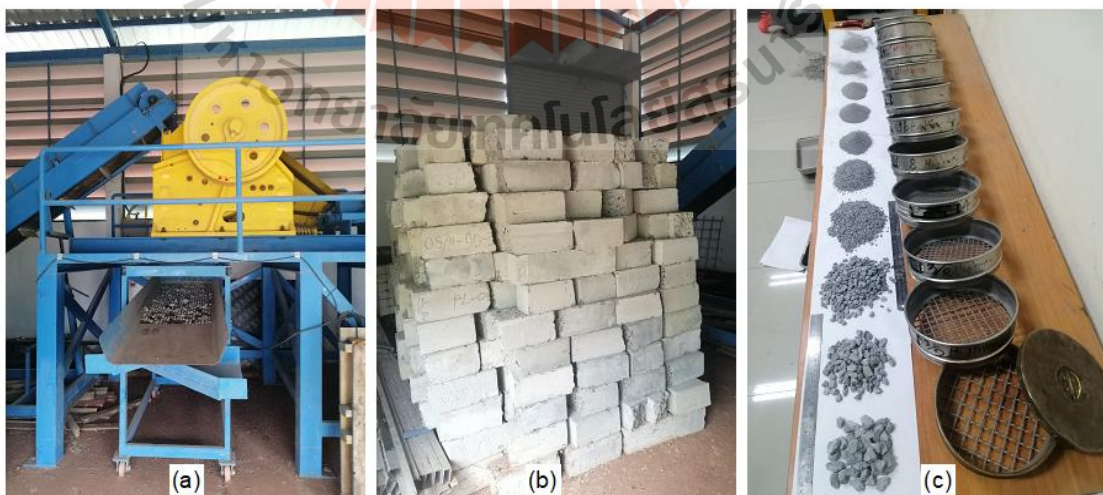
Figure 3.1 Photos: (a) concrete crusher machine, (b) concrete beams, (c) RCA particles.
