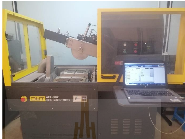
Figure 4.3 Hamburg wheel tracking device (HWTD) test setup.
