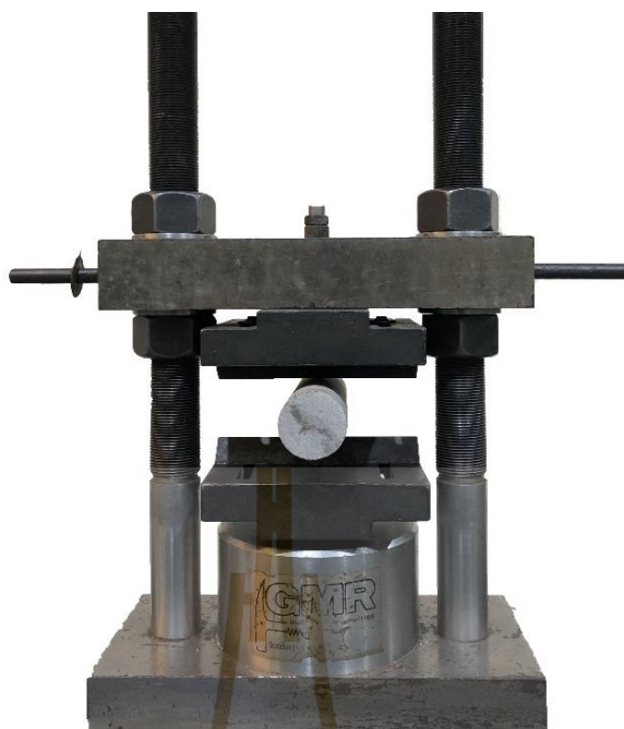
Figure 4.3 Creating an artificial fracture.
