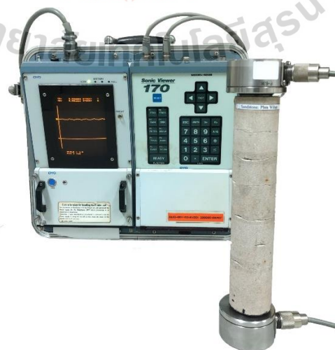
Figure 4.5 Some specimen of ultrasonic pulse velocity measurement.
